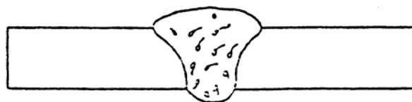
Porosity or Voids with Sharp Tails — None Acceptable
