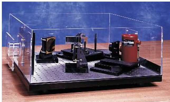
A grazing angle experiment, incorporating a photoelastic modulator for the analysis of thin films on metal
