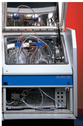
Figure 5. Agilent PL-GPC 220 integrated solvent delivery system
