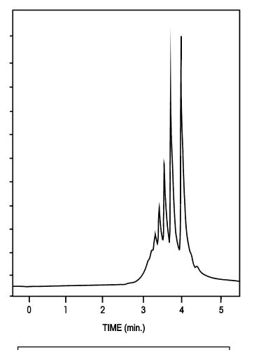
Conditions: Instrument: DuPont HPLC ZORBAX PSM 60S, 6.2 mm x 25 cm (Agilent P/N: 880957-802) Mobile Phase: Tetrahydrofuran; Flow Rate: 1.5 mL/min Temperature: 22°C; Detector: UV Abs (254 nm); Sample: Epon 836
