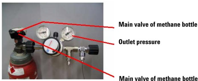
**Figure 32** Main valve and outlet pressure gauge
