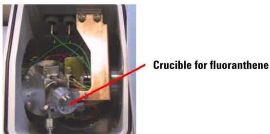
**Figure 40** Crucible for fluoranthene
