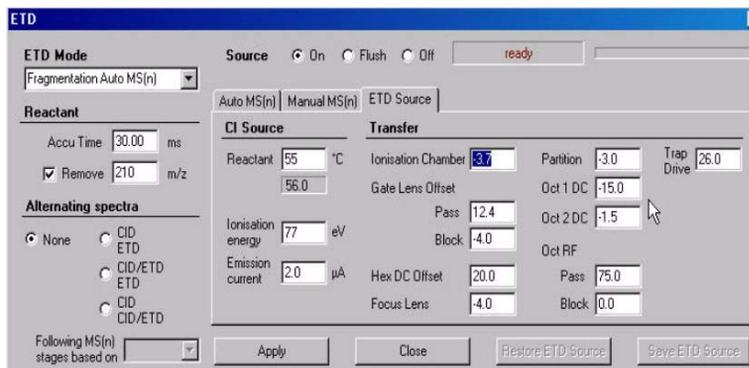
Figure 50 ETD source settings for proper ETD reactant ion formation.
