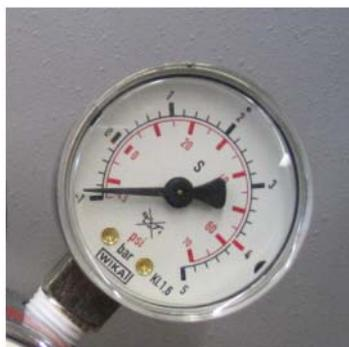
**Figure 39** Pressure gauge (low pressure stage) indicating about -0.8 bar (below ambient)
