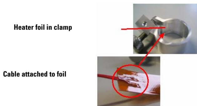
**Figure 17** Heater foil, cable, and clamp
