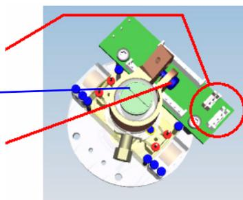
**Figure 15** Heater, temperature sensor plugs, and clamp
