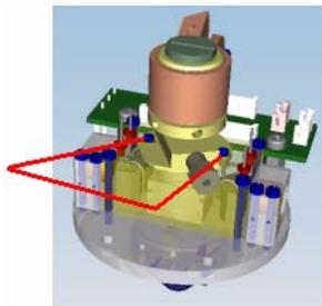
**Figure 23** Crucible retainer screws
