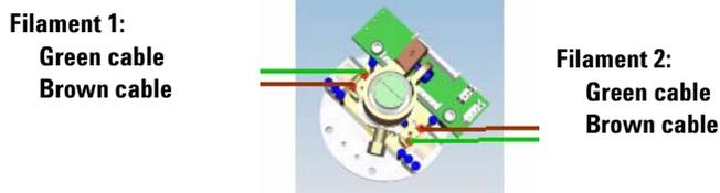
**Figure 26** Filaments and cable connections
