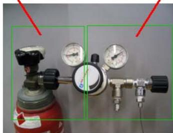
**Figure 35** High and low pressure stages of the methane gas supply
