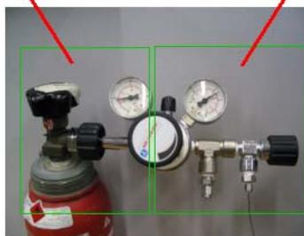
**Figure 30** High and low pressure stages of the methane gas supply
