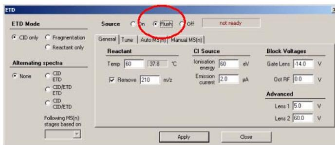
**Figure 37** ETD source Flush option (ETD dialog box)
