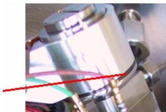
**Figure 19** Gap between heater device and crucible
