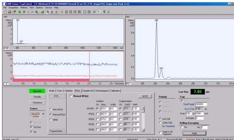
Figure 49 Proper appearance of the 202/203 reactant ions.
