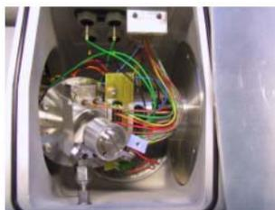
**Figure 20** Heater foil cables and nCI body
