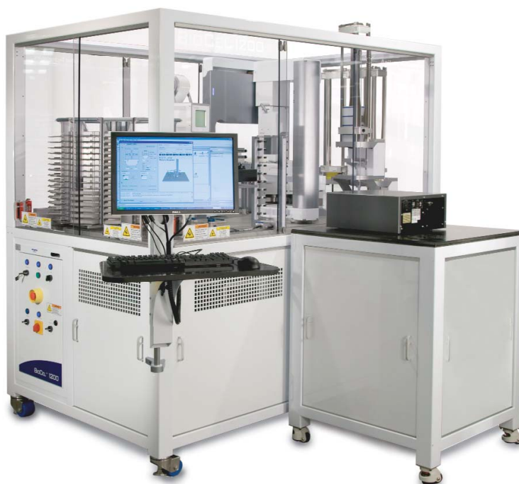
For additional flexibility and ease of access, the Direct Drive Robot can reach off the deck of the Agilent BioCel onto docking tables. Alternatively, the DDR itself can be placed on a docking table for outmost flexibility and mobility. Docking tables with QuickDock can be quickly moved and replaced without re-teaching the instrument position enabling instruments to be used offline when not in an automated protocol.
