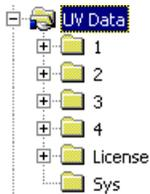
The installation of the UV-visible ChemStation Security Pack on the Server will create the UV-visible instruments data structure for four instruments on the shared ChemStation directory, as specified in step 6. Four subdirectories named 1,2,3, and 4, are created as four instruments can be connected to one ChemStation. On the next level you will find the directories for methods, data etc., where the ChemStation data will be saved.
