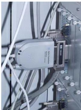
**Figure 7** USB-GPIB Interface Connection
