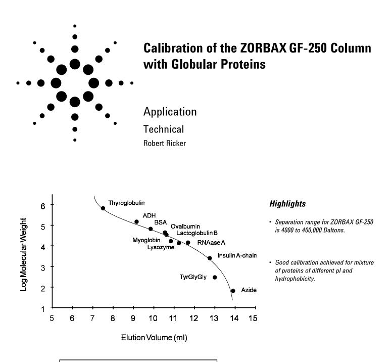
Conditions: ZORBAX BioSeries GF-250 9.4 x 250 mm (Agilent P/N: 884973-901) Mobile Phase: 0.2 M NaH<sub>2</sub>PO<sub>4</sub>, pH 7.0 Detection: UV 230 nm
