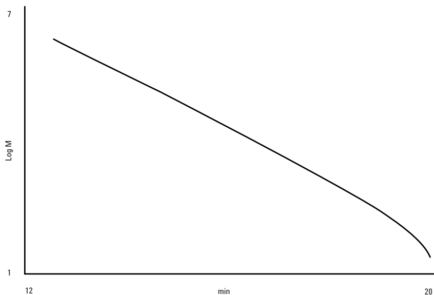
Figure 8. PL aquagel-OH MIXED-H 8 \mu m column calibration using PEO EasiVial standards showing the relationship between retention time and the log of molecular weight
