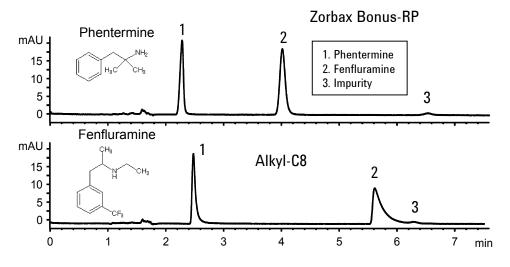
**Conditions:** HPLC System: Agilent 1100 with quaternary pump Column: ZORBAX Bonus-RP,  $4.6 \times 150$  mm, Agilent P/N: 883668-901 Mobile Phase: [MeOH: ACN (50:50)]:  $K_2HPO_4$ , 25 mM, pH 7.2, (55:45) Detector: UV 254 nm; Flow: 1 mL/ min.; Temperature: ambient
