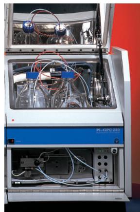
Figure 5. Agilent PL-GPC 220 integrated solvent delivery system
