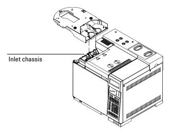
2. Tighten the three captive screws. Install the three M4×67 screws and tighten until snug.
