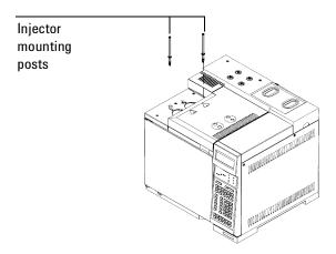
3. Remove the inlet cover. Loosen the 6 captive screws with a T-20 Torx screwdriver until you are able to lift off the cover.
