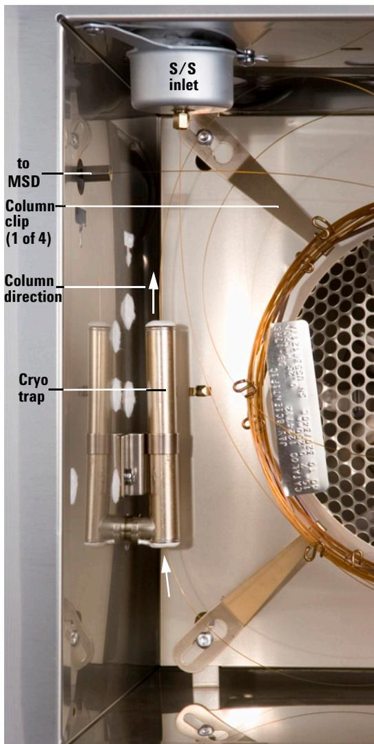
**Figure 38** Routing Column 2 through the cryo trap
