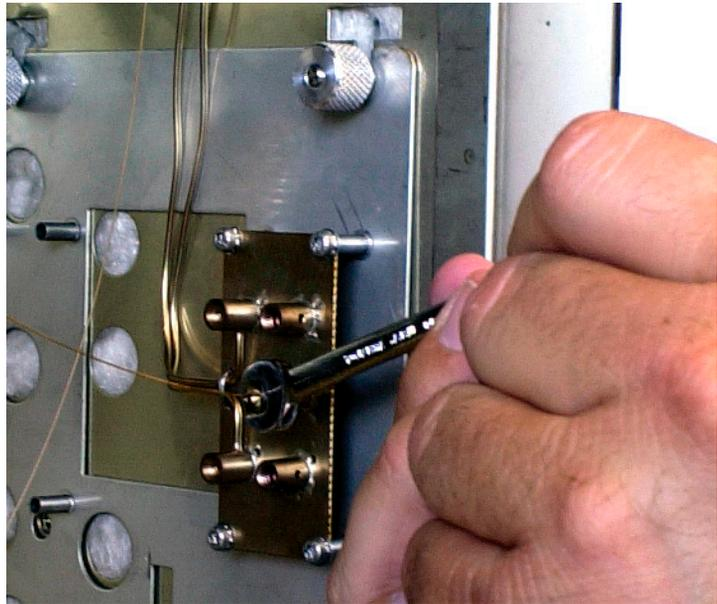
**Figure 41** Tighten the fitting nut by no more than 15 to 20 degrees
