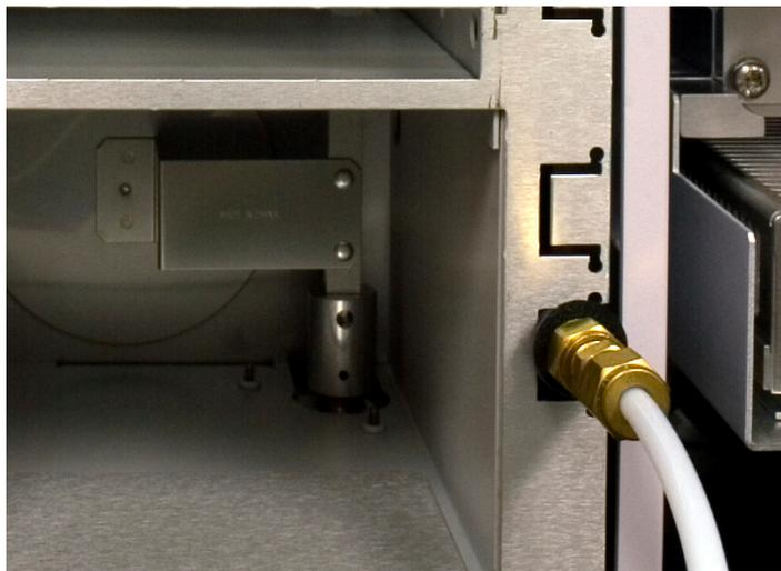
**Figure 6** Air connection to Cryo Trap
