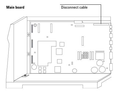
4. From the pneumatics carrier, locate the ribbon cable you unplugged in Step 2 and pull it through the slot.
