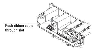
9. From the main board, locate the EPC board connector on the upper right-hand side. Make certain connector is in the open position. Plug the ribbon cable into the connector and push until the plug is firmly in place. Lock the connector by moving the tabs to the center of the connector until they click into place.
