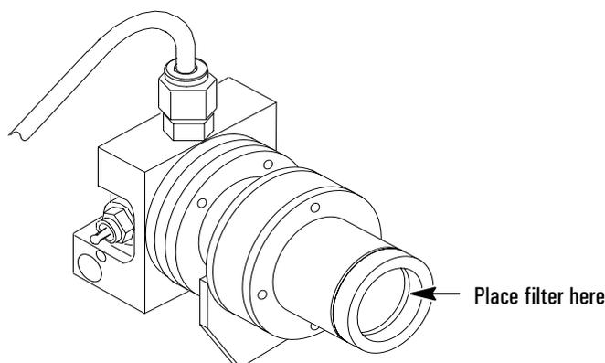
6. Push the PMT housing as far onto the detector body as it will go.
