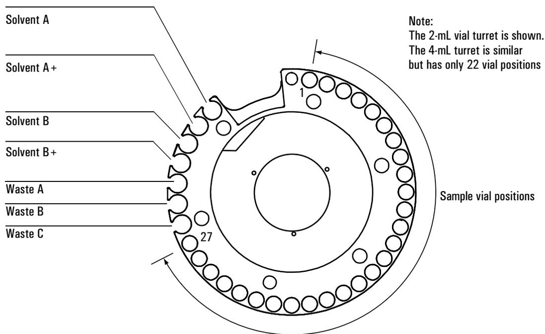
**Figure 47. The 6850 Automatic Liquid Sampler turret (2-mL version shown)**
