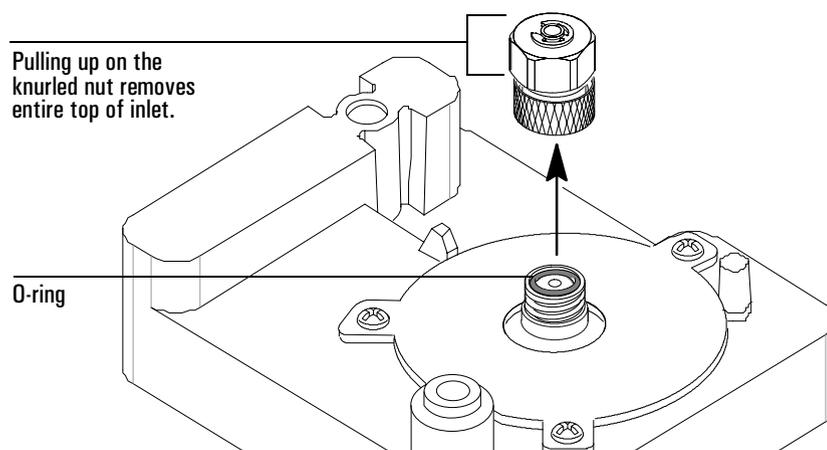
4. Replace the top portion of the inlet and tighten the knurled nut until you cannot tighten it further. Restore the GC to normal operating conditions.
