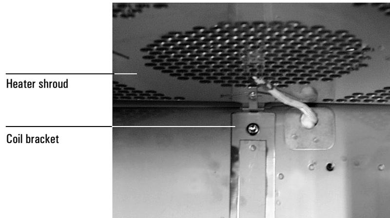
2. Place the cooling coil in the oven with the fitting at the upper left. The bottom center of the coil should rest on the coil bracket.
