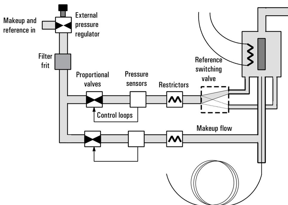
Figure 31. Internal/External TCD plumbing
