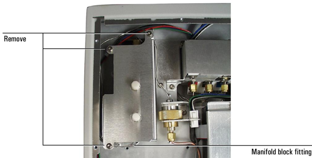
9. If your 6850 has a valve box installed, remove the valve box cover.
