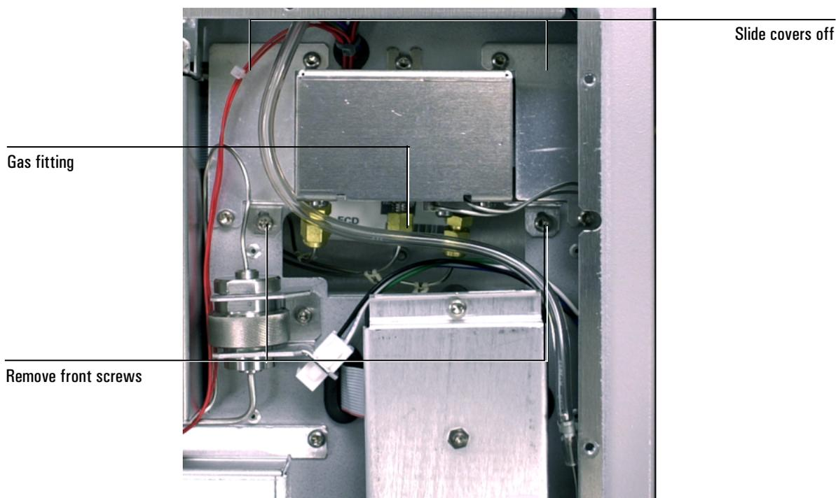
**Figure 35. Removing the flow module**
