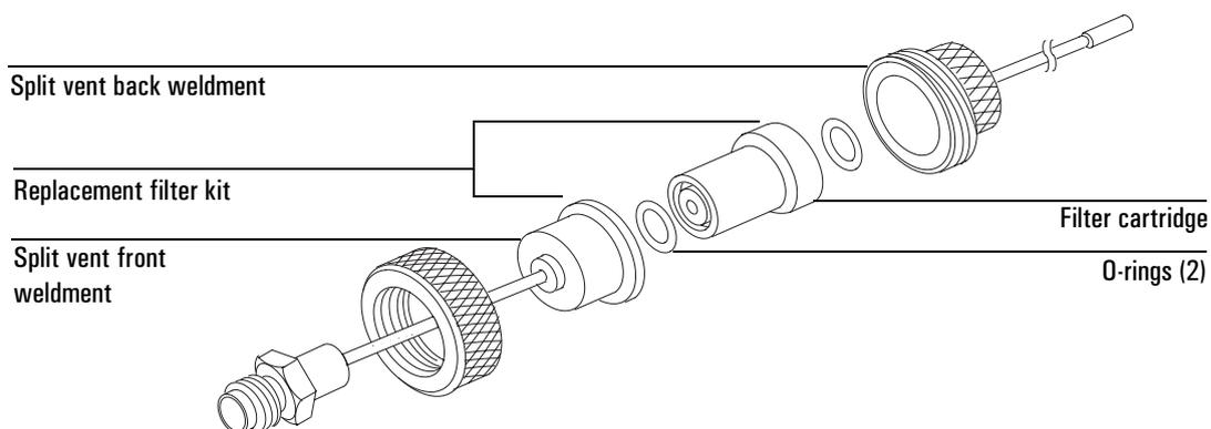
5. Replace the two O-rings and filter cartridge.
