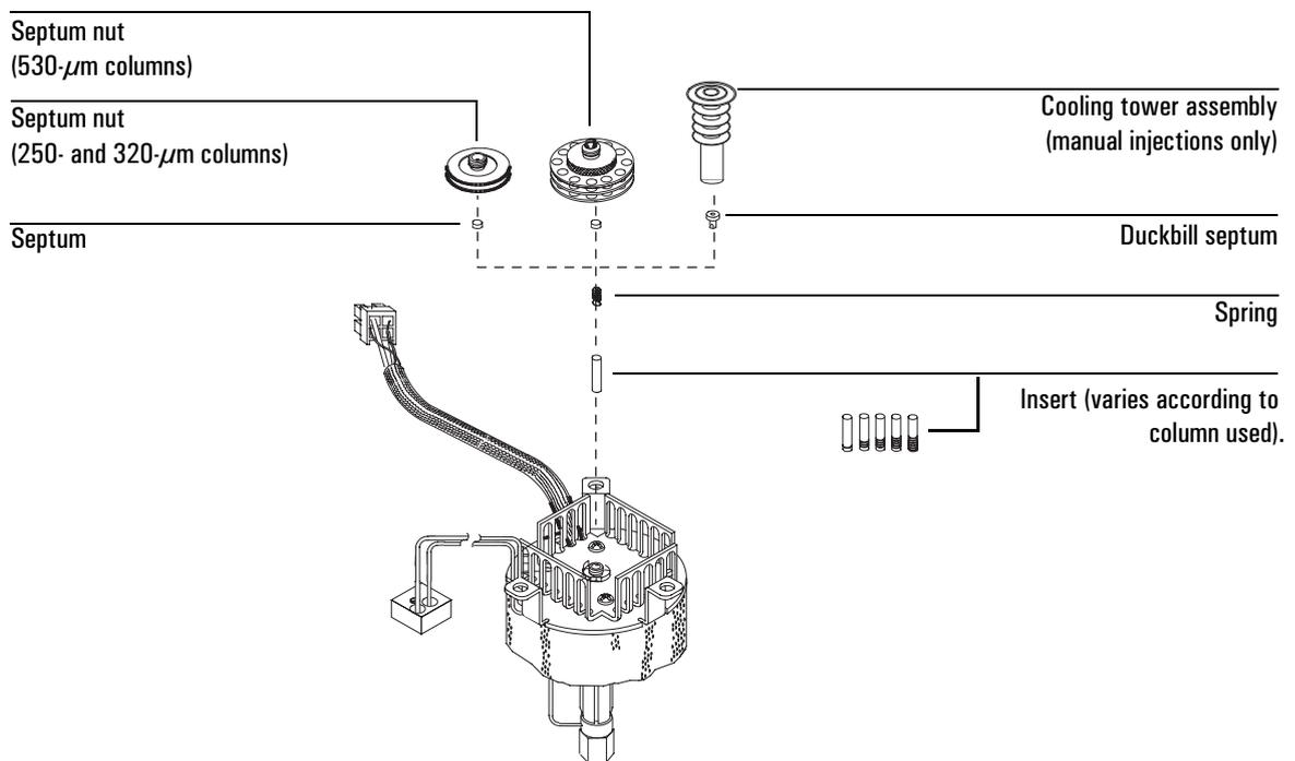
**Figure 30.** The cool on-column inlet
