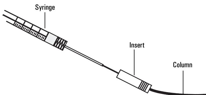
3. Insert the syringe needle through the other end of the insert and into the column. If the needle cannot pass easily into the column, reverse the insert to try the needle and column in the other end.
