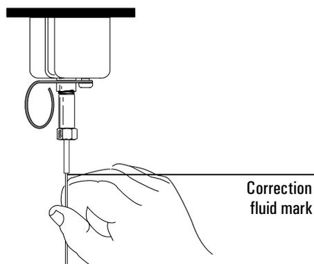
7. Tighten the column nut an additional 1/4 to 1/2 turn so that the column cannot be pulled from the fitting when gentle pressure is applied.
