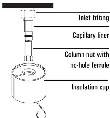
2. Install the insulation cup, if needed. Push the cup spring to the right. Slide the cup over the inlet fitting so that the insulation at the top of the cup is flush against the oven roof.
