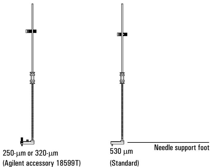
**Figure 45. Needle support assembly**
