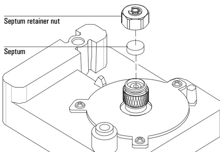
If the septum sticks, use a sharp-tipped tool to remove it. Take care not to gouge the metal around the septum and make sure you remove all pieces of the old septum.
