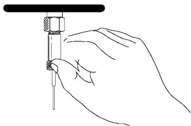
3. Tighten an additional 1/4-turn with a wrench or until the column does not move.
