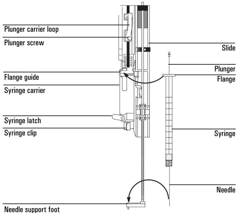
**Figure 42. Installing the syringe**
