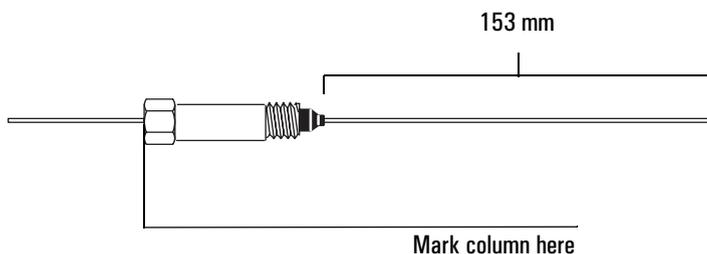
6. Insert the column in the detector. Slide the nut and ferrule up the column to the detector base. Finger tighten the column nut until it starts to grab the column.
