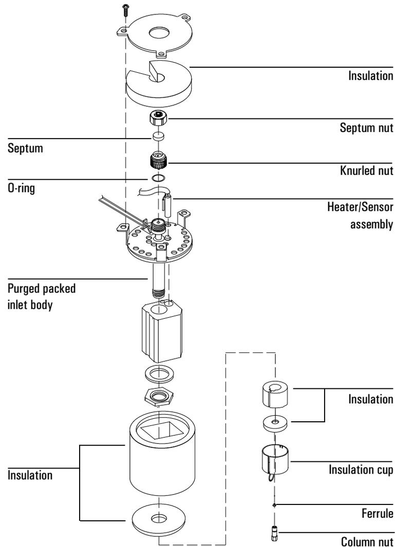
**Figure 26. The purged packed inlet**
