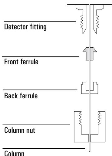
See [Table 13](#) for the proper ferrules. Trim off a short piece of column to remove any ferrule fragments inside the column.
