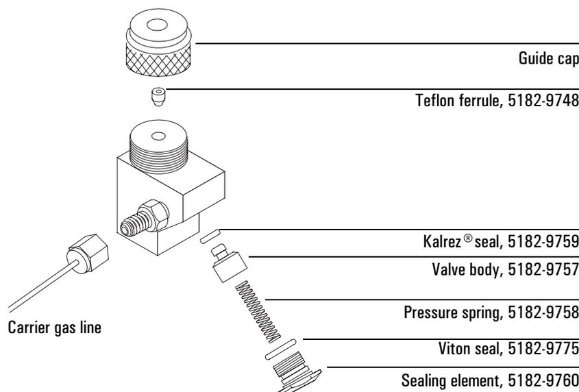
4. Unscrew the guide cap from the head and remove the Teflon ferrule.
