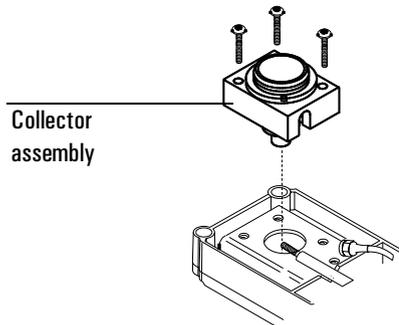
7. Using the nut driver, loosen the jet and pull it straight out. You may need to use the forceps to grasp the jet.
