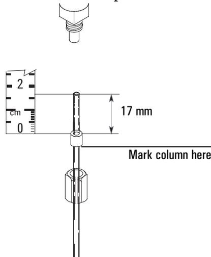
7. Screw the column nut on finger tight. Using a 5-mm wrench, tighten the column nut 1/8- to 1/4-turn. Be careful not to overtighten.
