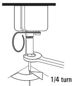
8. After the column is installed at both inlet and detector, establish a flow of carrier gas through the inlet. Heat the oven, inlet, and detector to operating temperatures. Allow these to cool, and then retighten the fittings.
