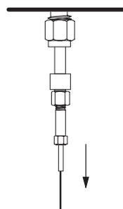
7. Use a wrench to tighten the nut an additional 1/4 turn.
