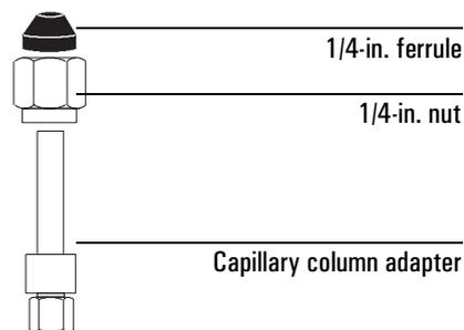
2. Insert the adapter straight into the detector base as far as possible. Hold the adapter in this position and tighten the nut finger tight. Use a wrench to tighten the nut an additional 1/4 turn.
