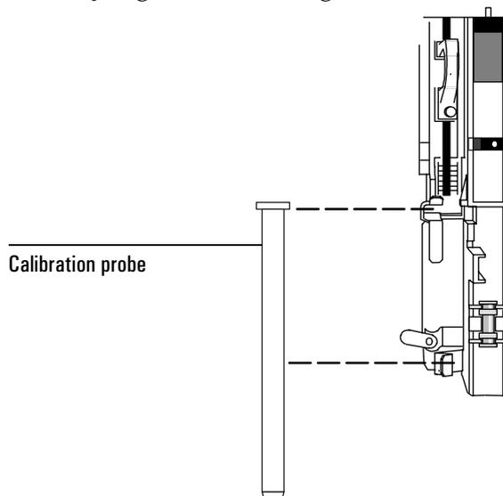
6. When alignment is complete, the green light will be on if the injector door is closed, or the red light will be on if it is open. Remove the calibration probe and secure it in its clamps below the turret.
