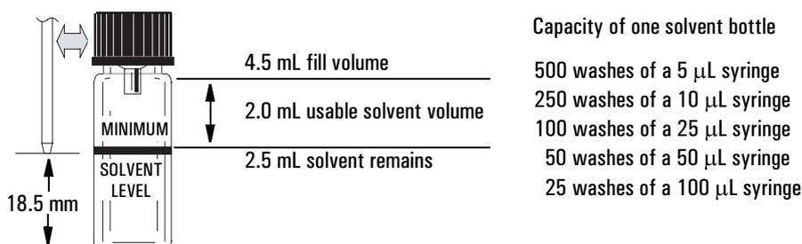
**Figure 39. Position of syringe tip when withdrawing solvent**
