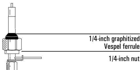
2. Prepare the column. See “Installing capillary columns” on page 27 for instructions.
