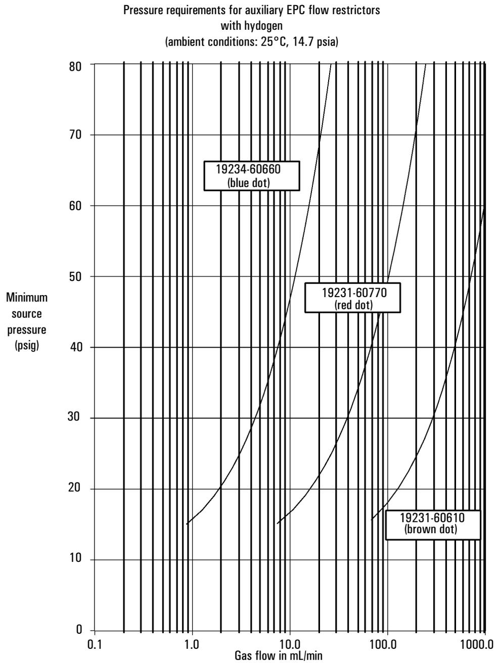
**Figure 24. Pressure requirements for auxiliary EPC flow restrictors with hydrogen**
