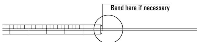
**Figure 41. Syringe needle inspection**
