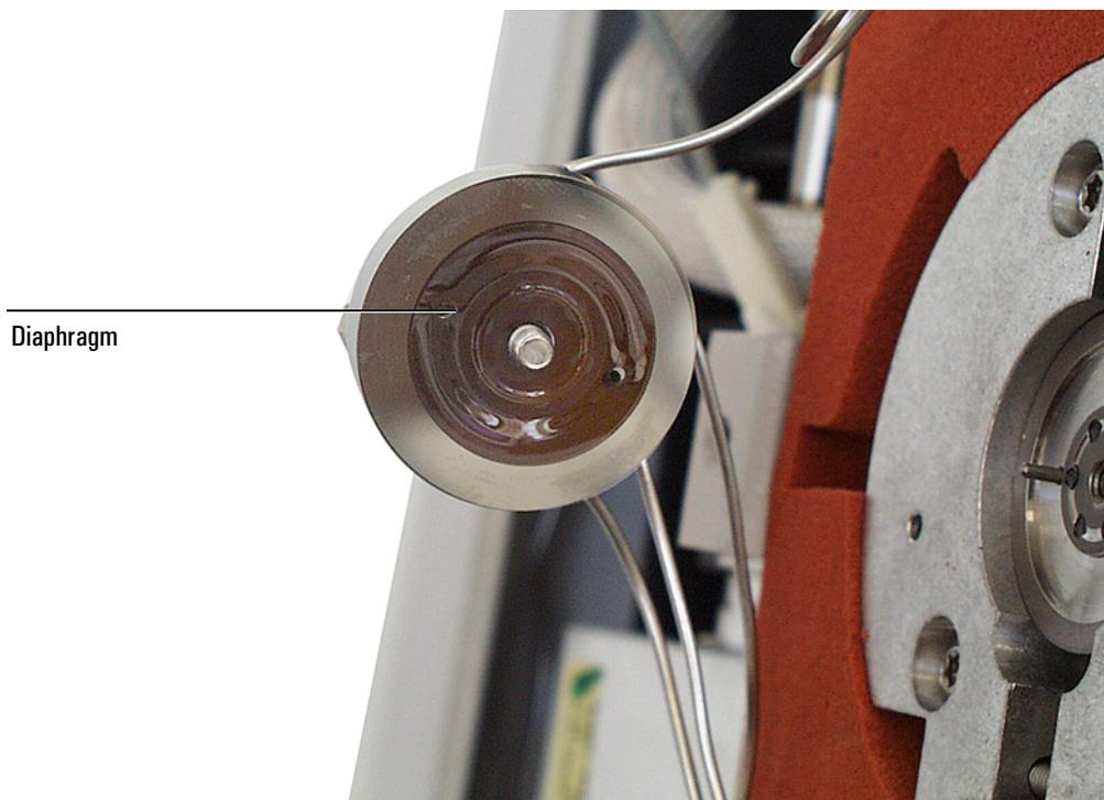
9. Align the new diaphragm over the mounting posts so that the valve diaphragm channel is oriented toward the shiny valve face.
