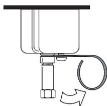
3. Place the spring into the groove in the inlet liner. Remove the column nut and put the no-hole ferrule aside.
