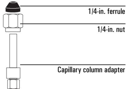
2. Insert the adapter straight into the detector base as far as possible.
