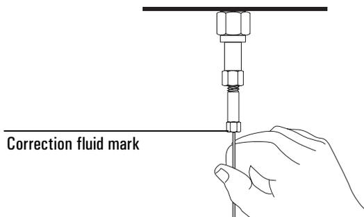
8. Tighten the column nut finger tight, then withdraw the column about 1 mm. Use a wrench to tighten the nut an additional 1/4 turn.
