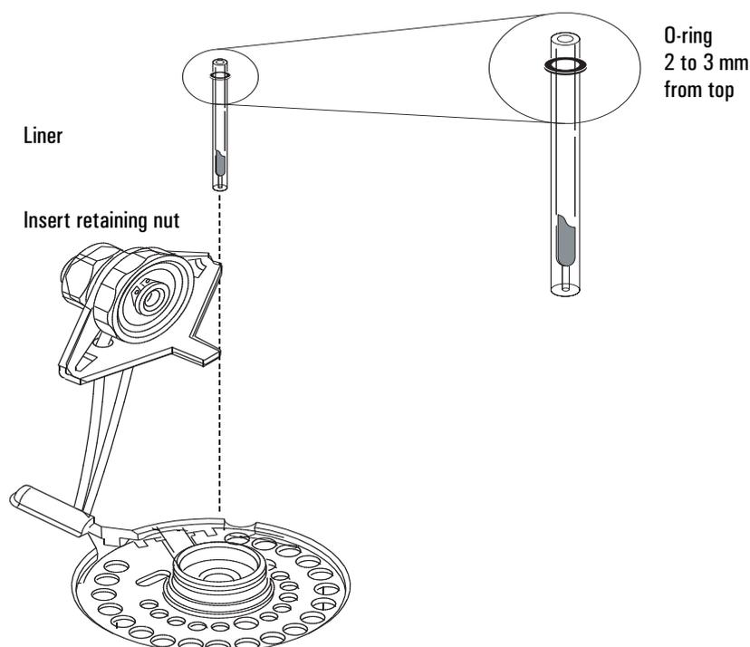
**Figure 25. Installing a liner**
