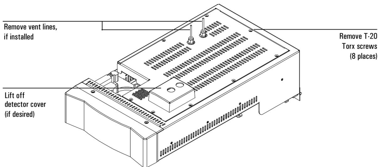
Lid top cover for FID/TCD/ $\mu$ ECD, without valve box accessory, is shown
