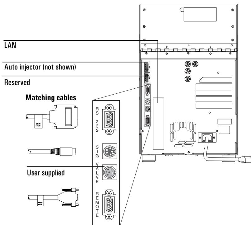
**Figure 3. Electrical connections**
