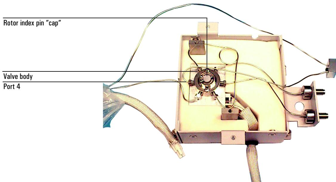
**Figure 20. Valve body in valve box**
