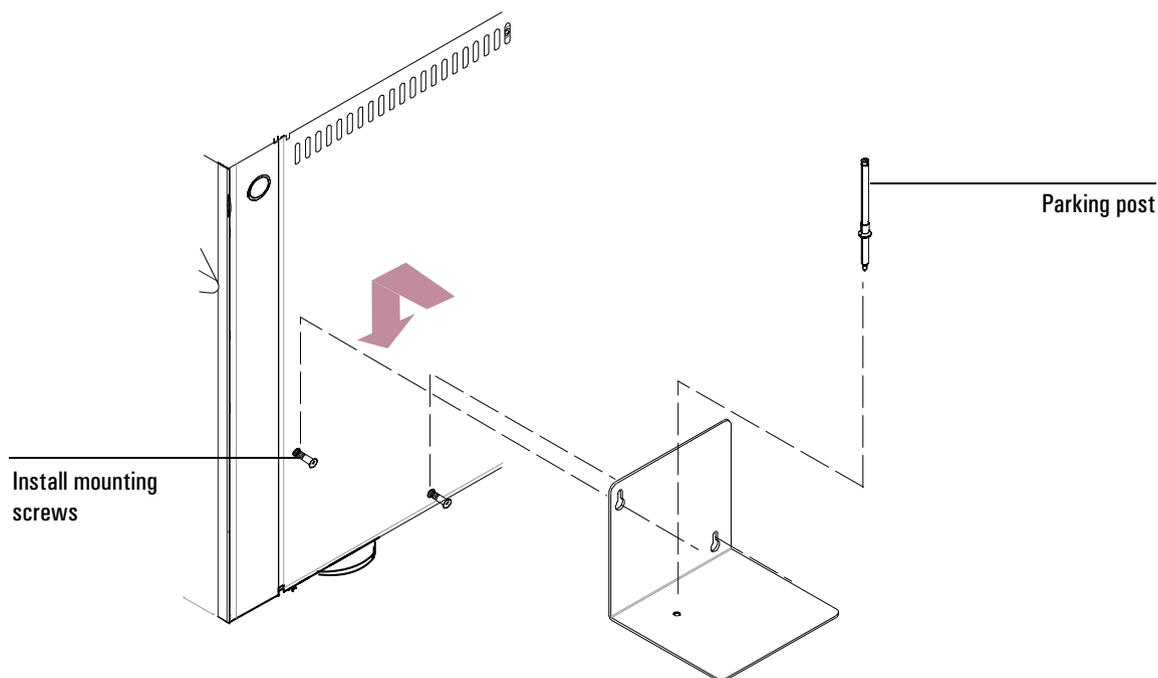
**Figure 53.** Installing the injector mounting bracket on the side of the GC
