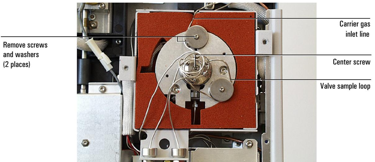
6. Loosen the sample loop's two 1/4-inch fittings on the valve head and lift the loop away from the instrument.
