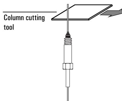
3. Support the column end against the column cutter opposite the scribe and break off the end. Inspect the end with a magnifying glass to make certain there are no burrs or jagged edges.
