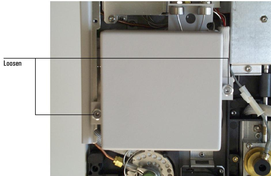
5. Remove the two screws and washers that hold down the valve sample loop and the carrier gas inlet line.
