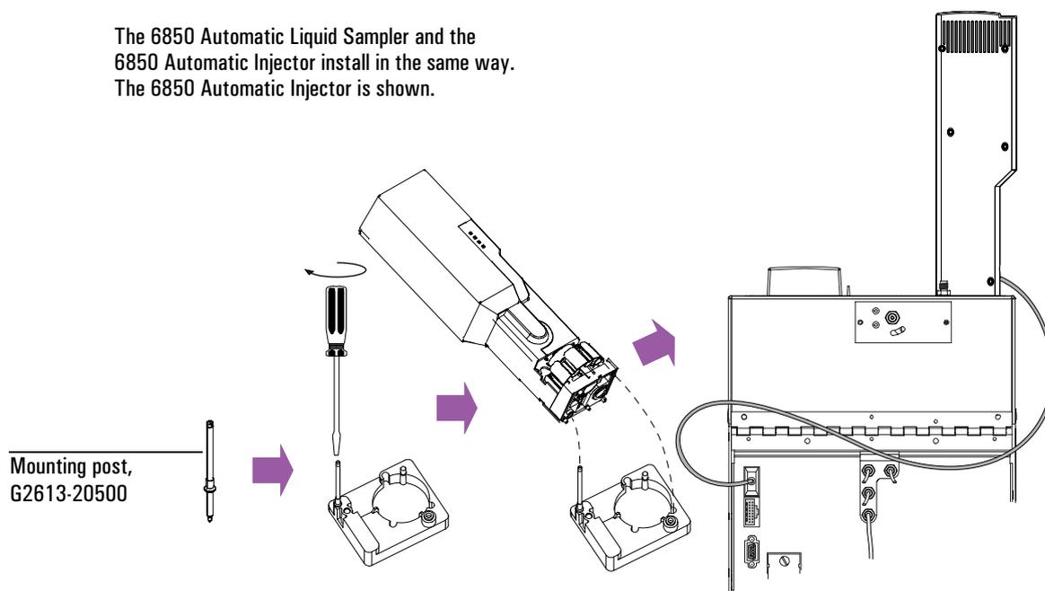
**Figure 52.** Installing the mounting post and mounting the injector
