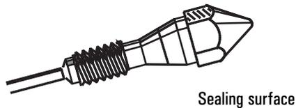
9. Inspect the jet tube to make sure it is not bent or crimped. Inspect the jet for contamination or pieces of broken column by holding it up to a light and looking through it. If no contamination is present, the tube will be clear.
