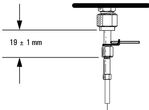
5. Slide the nut and ferrule up to the detector fitting and tighten the nut finger tight. Use a 9/16-inch wrench to tighten the nut an additional 1/4 turn.
