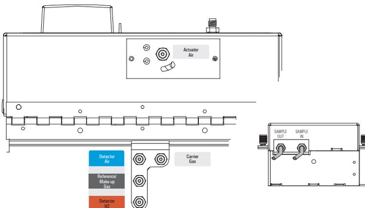
**Figure 2. Gas connections**
