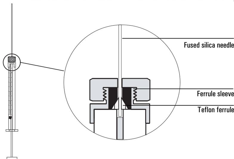
3. When the needle is inserted, tighten the retaining nut to *firm* finger tightness. Pull the needle gently to be sure the Teflon ferrule has formed a tight seal with the needle. Tighten the retaining nut further, if necessary.
