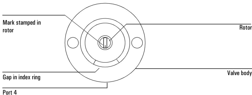
**Figure 21. Top of rotor aligned towards port 4**
