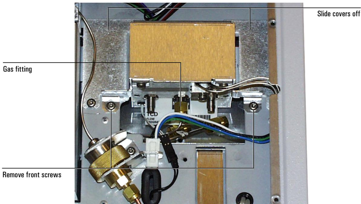
8. Unscrew the manifold block fitting from the flow module.
