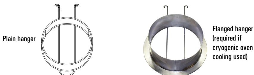
**Figure 5. Capillary column hanger**
