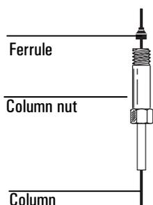
2. Score the column using a column cutting tool. The score must be square to ensure a clean break.
