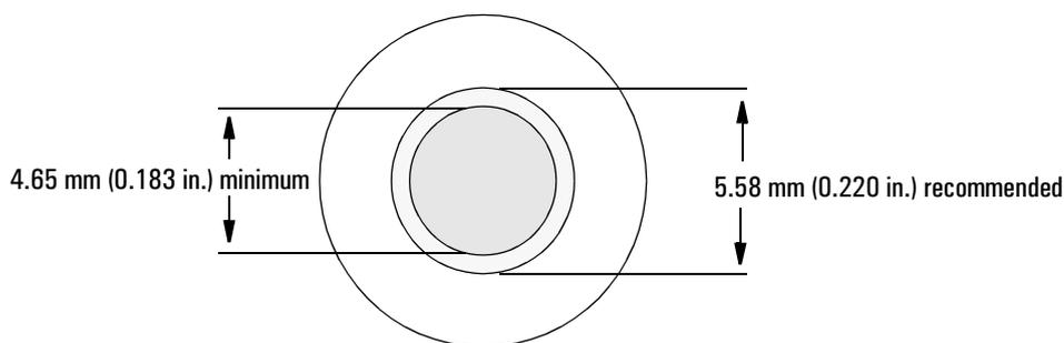
**Figure 38. Vial cap aperture specifications**
