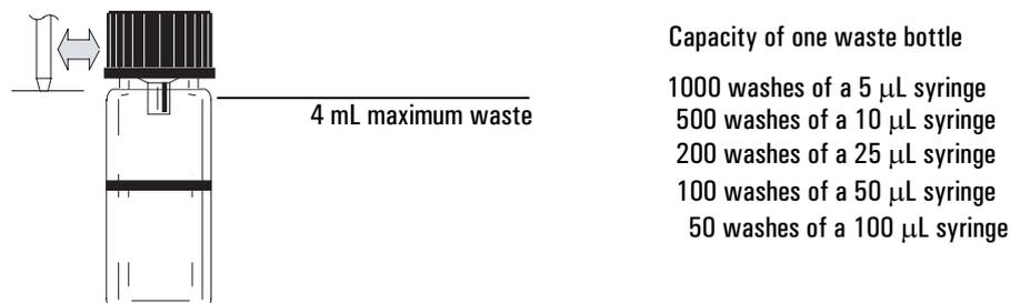
**Figure 40. Position of syringe tip when discarding waste**
