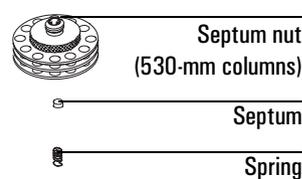
Make sure the spring is in the inlet. Use the tweezers to place a new septum on the bottom of the septum nut, and then reattach the septum nut to the inlet. Tighten the nut firmly.
