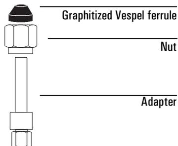
2. Insert the adapter straight into the detector base as far as possible. Hold the adapter in this position and tighten the nut finger tight.
