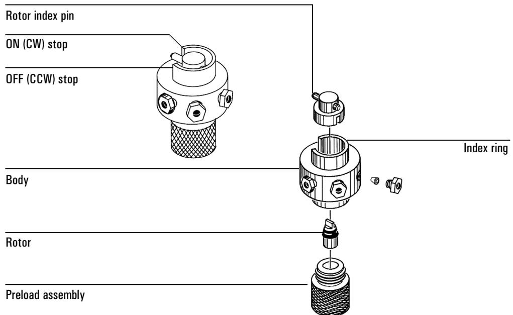
**Figure 16. A typical 6-port rotary valve**
