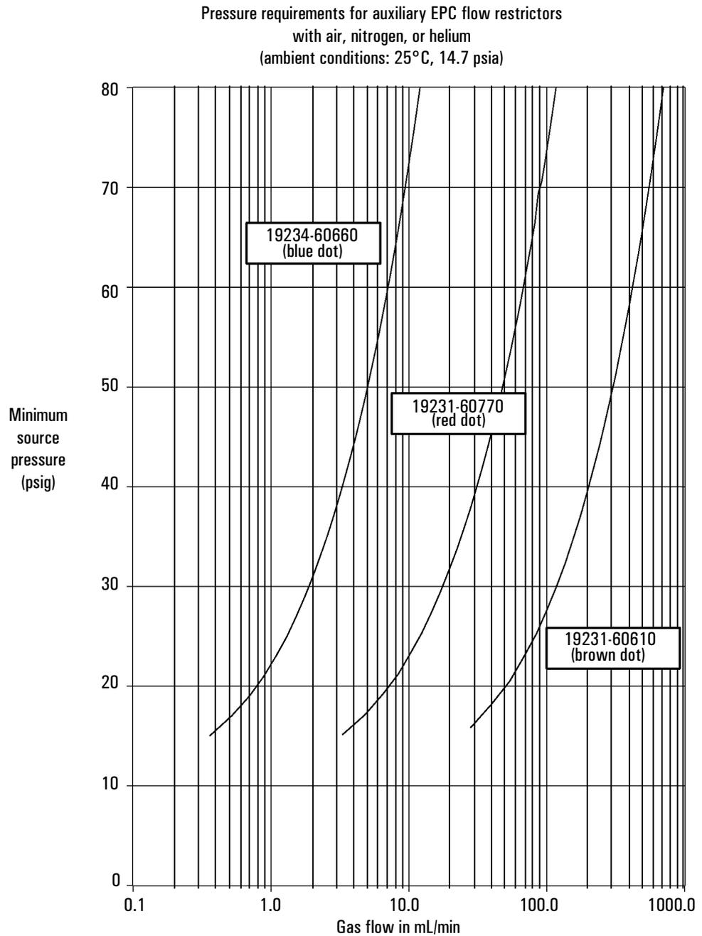
**Figure 23. Pressure requirements for auxiliary EPC flow restrictors with air, nitrogen, and helium**
