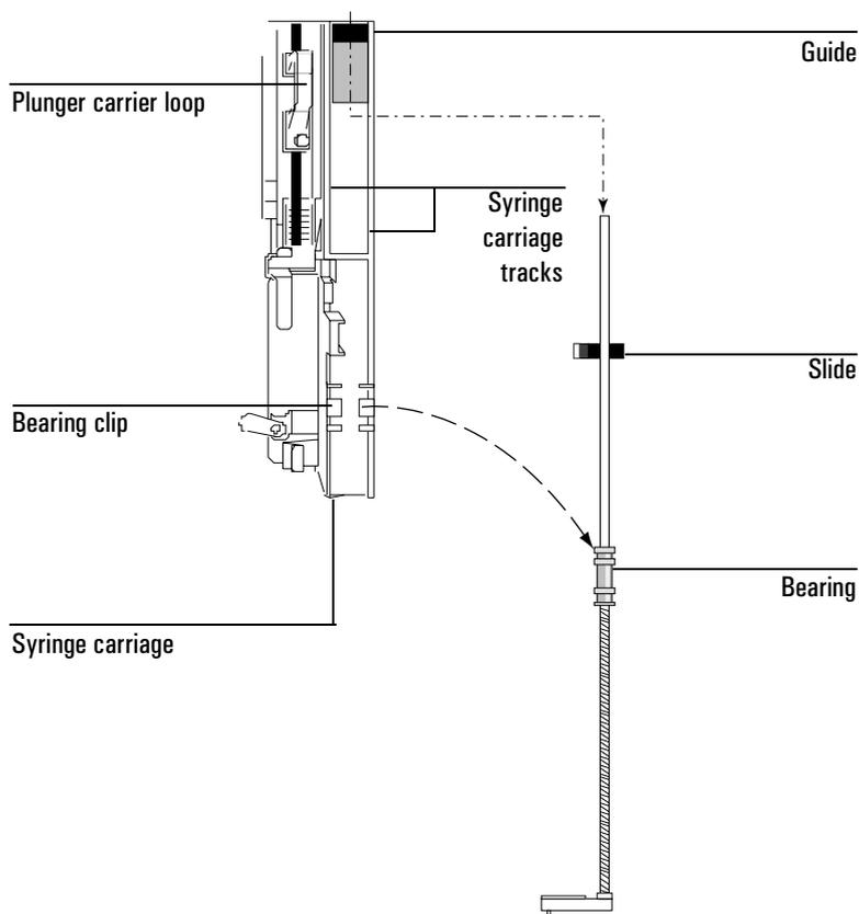
**Figure 44. Removing the needle support assembly**
