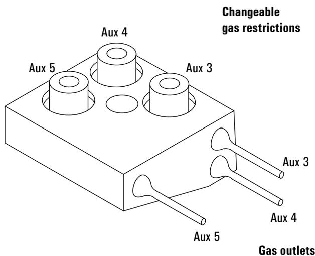
5. Pull the frit to be changed out of the block. Also remove the O-ring that seals it.
