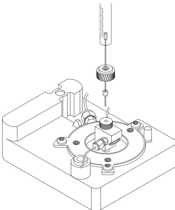
3. Push the guide cap and the new Teflon ferrule over the syringe needle so that at least 10 mm of the needle tip is exposed.
