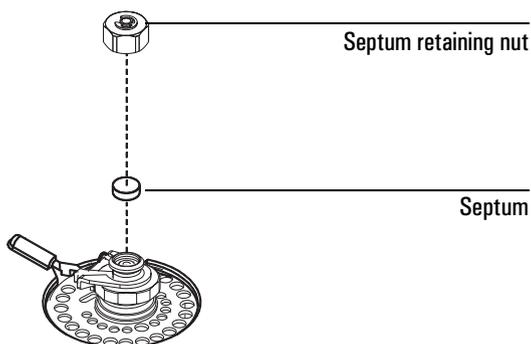
4. If pieces of the septum stick, use a small piece of rolled-up steel wool and forceps or tweezers to scrub the residue from the retainer nut and septum holder. Use compressed air or nitrogen to blow away the debris.
