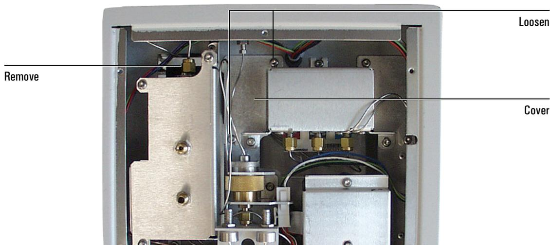
5. Slide the cover plate off to expose the ribbon cable.
