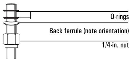
2. Insert the column into the inlet until it bottoms. Insert the column into the detector fitting but do not force it. It may be necessary to start the long end of the column in the inlet at an angle.
