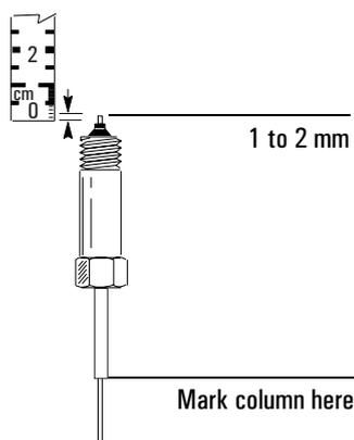
6. Push the column up 1 cm and guide it into the inlet liner. Slide the nut and ferrule up the column to the inlet liner. Adjust the column position so that the correction fluid mark on the column is even with the bottom of the column nut. Finger tighten the column nut until it starts to grab the column.
