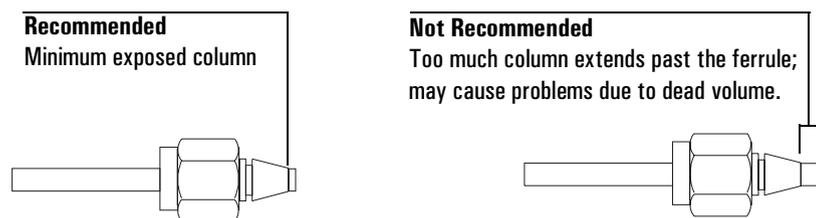
Use the following instructions to install new SWAGELOK® nuts and ferrules onto 1/8-in. or 1/4-in. metal columns.
