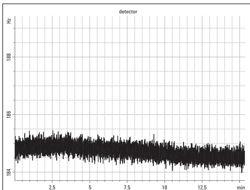
**Figure 10. Sample  $\mu$ ECD noise, wander, and drift plot**
