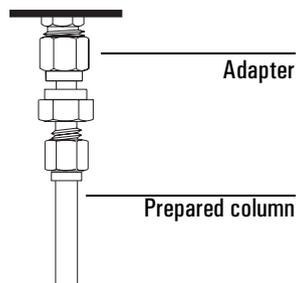
2. If you are installing a column directly into the detector fitting:
