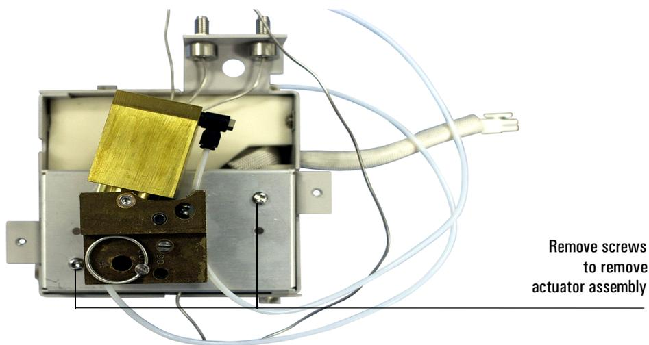
**Figure 19. Removing the valve actuator assembly from the valve box**
