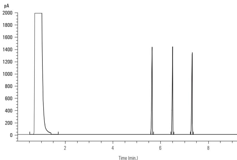
**Figure 9. Sample FID checkout chromatogram**
