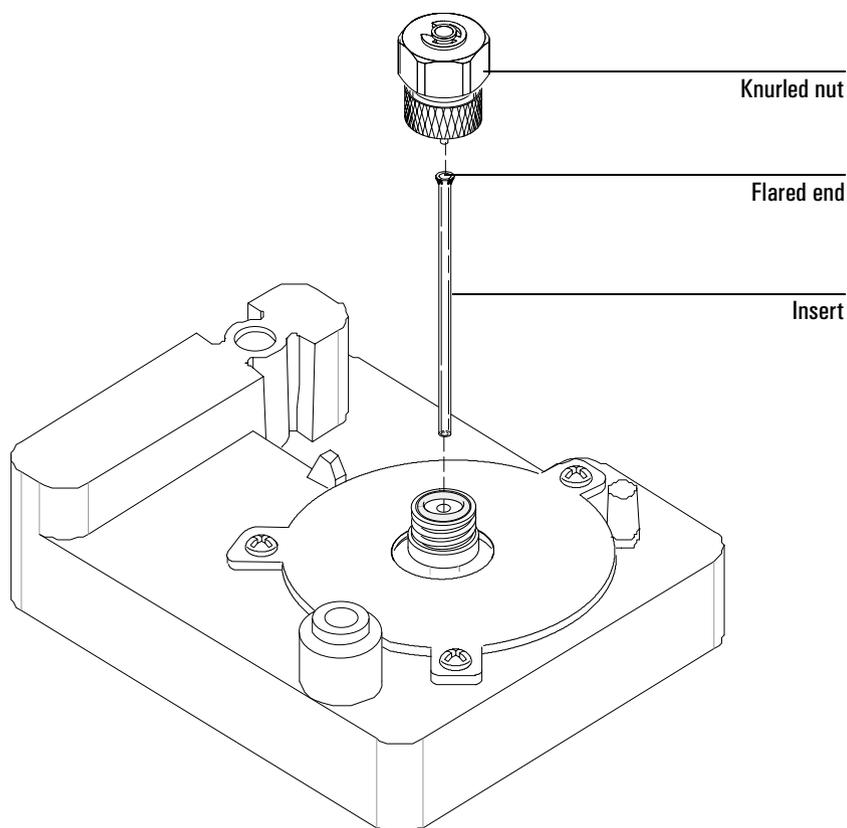
**Figure 28. Installing a glass insert in a purged packed inlet**
