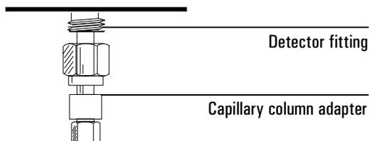
3. Install a column nut (part no. 18740-20870) and graphite ferrule (1.0 mm id, part no. 5080-8773 or 0.5 mm id, part no. 5080-8853) on the column.
