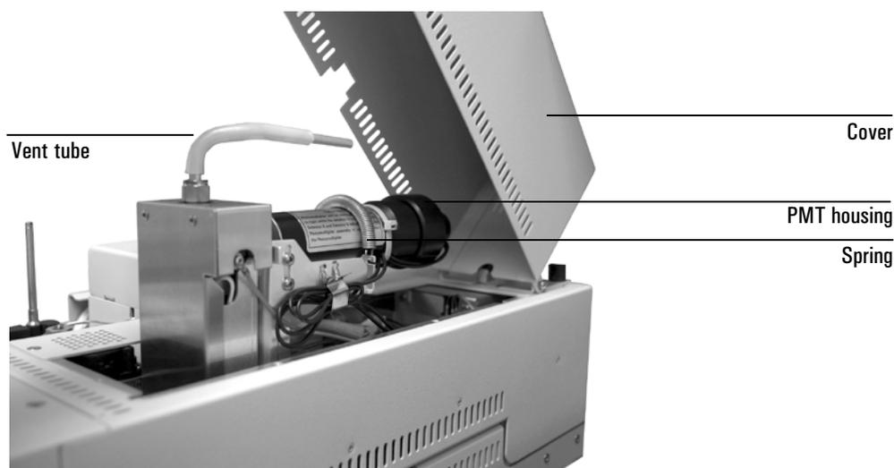
2. Release the retaining spring around the photomultiplier housing.
