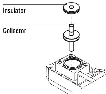
6. Remove the three screws that hold the collector bottom assembly in place. Lift off the assembly. Remove the lower insulator from the bottom assembly. You may need to use the forceps to grab it.
