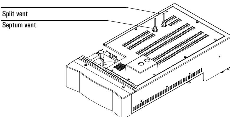
**Figure 29. Capping the bottom of the inlet and septum purge vent**
