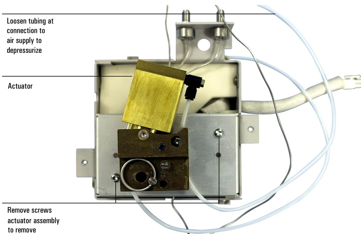
**Figure 17. Rotary sampling valve actuator air supply**
