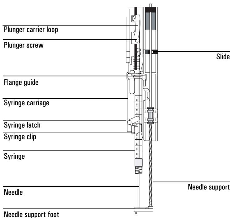
**Figure 43. Syringe carriage and needle support with needle installed**
