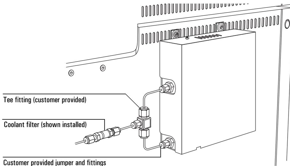
**Figure 55. Cryo coolant fittings**
