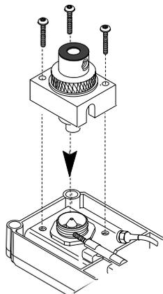
11. Install the column and restore normal operating conditions.
