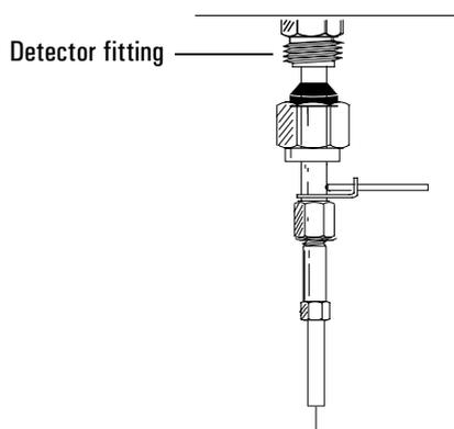
If the adapter is properly installed, the distance between the 1/4-inch nut and the bottom of the adapter will be  $19 \pm 1$  mm. If it is 22 to 23 mm, reinstall the adapter into the detector fitting.
