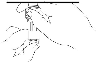
4. Place the ferrule and column nut on the column end. Trim off a short piece to remove any ferrule fragments inside the column.
