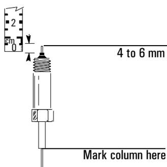
3. Insert the column in the inlet and slide the nut and ferrule up the column to the inlet base. Finger tighten the column nut until it starts to grip the column.
