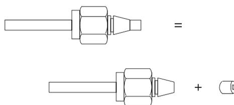
6. Insert the spacer into the vise-held Swagelok fitting.
