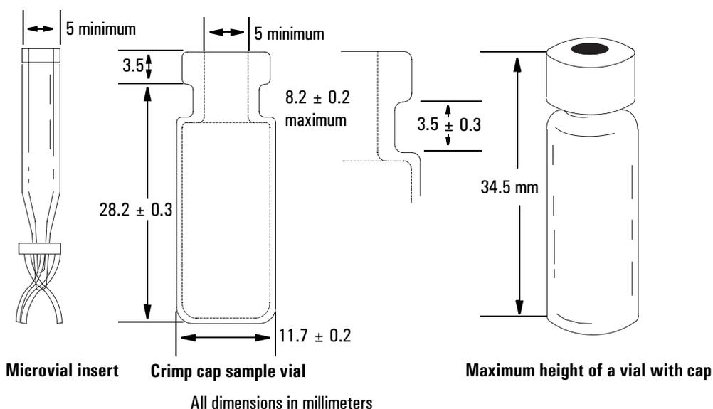
**Figure 36. Dimensions for sample vials and microvial inserts**
