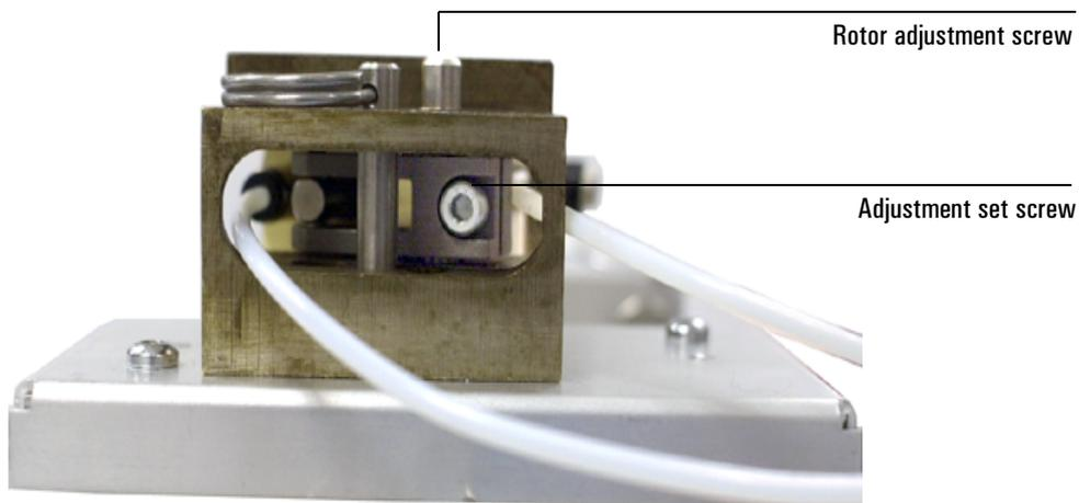
**Figure 18. The adjustment set screw**
