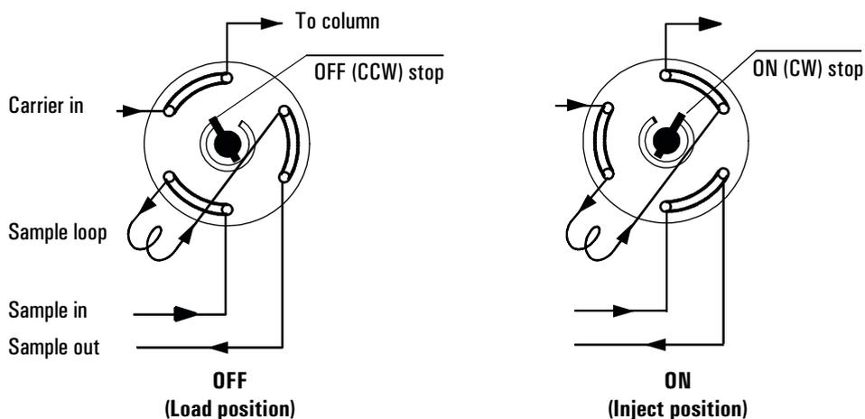
**Figure 22. Gas sampling valve plumbing**
