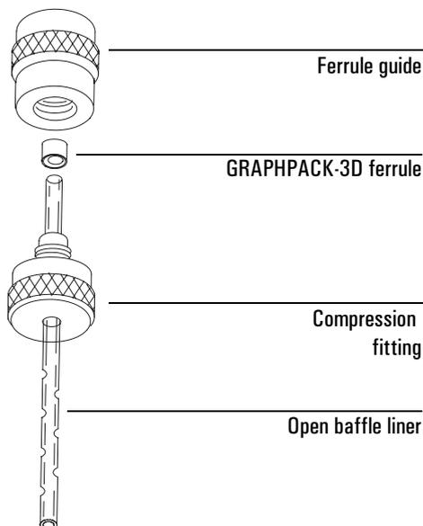
4. Slide the compression fitting onto the longer straight end of the new liner with the threads pointing toward the end of the liner.
