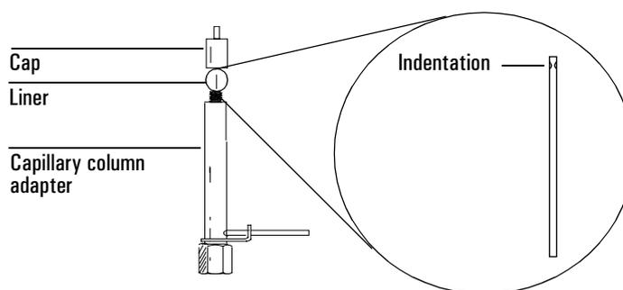
**Figure 34. The  $\mu$ ECD adapter**
