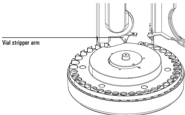
6. To remove the turret, lift the turret straight up to free it from the motor hub.
