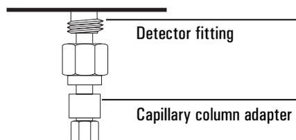
3. Hold the adapter in this position and tighten the nut finger tight. Tighten 1/4 turn more with a wrench.
