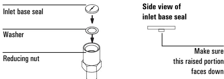
6. Replace the reducing nut and tighten with a wrench. Replace the column and the insulation cup. After the column is installed, you can restore normal operating conditions.
