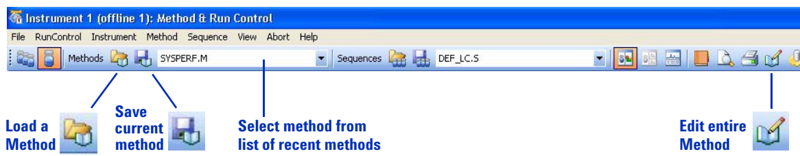
Figure 19 When you click the icon for the Single Sample Toolset , you access tools to work with methods.
