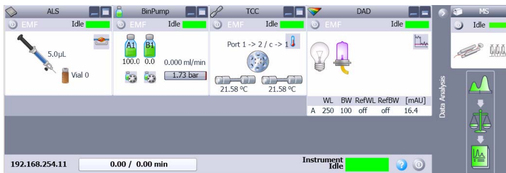
Figure 22 You can right-click a module in the system diagram to access context menus that allow you to change settings.
