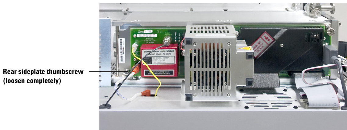
Figure 5 Loosen sideplate thumbscrews
