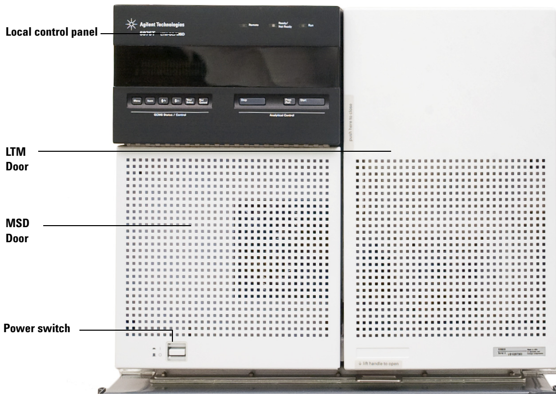
Figure 1 5975T LTM GC/MSD system
