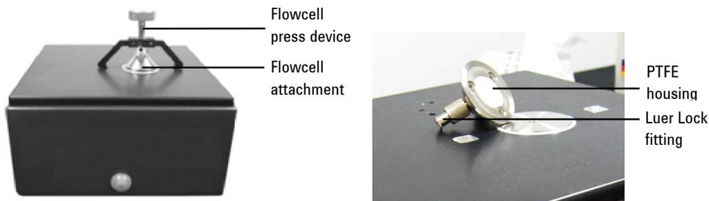
**Figure 10.** Nine reflection ATR flowcell attachment
