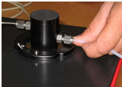
**Figure 14.** Attaching the purge gas hose to the gas cell inlet
