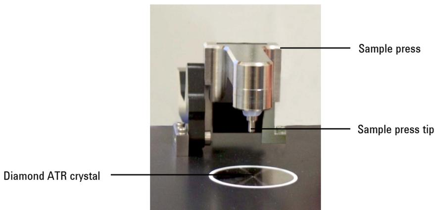
**Figure 7.** Sample press in highest position providing easy access for sample loading and cleaning
