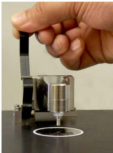
**Figure 9.** Opening the sample press
