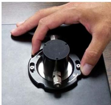
**Figure 13.** Attaching the gas cell
