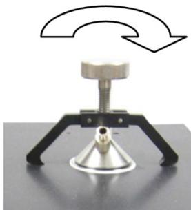
**Figure 11.** Securing the flowcell press device
