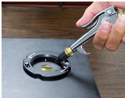
**Figure 12.** Cleaning the sample interface
