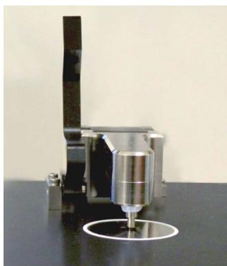
**Figure 8.** Sample press lowered for analysis
