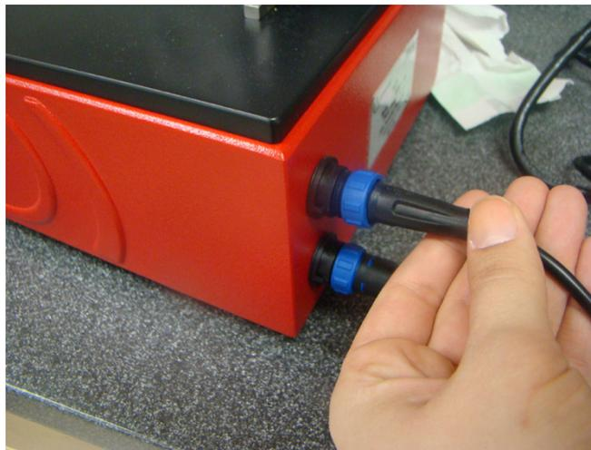
**Figure 3.** Attaching the USB cable
