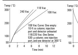
Gradients (temperature variations within a column) Specification: less than 2 °C within a 9-in. coil anywhere within the operating range
