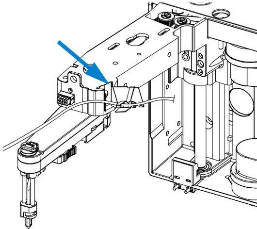
**5** Unplug the capillary assembly from the bolt carrier (located on the top center of the front cover) by moving the snapper as indicated by the arrows. Slide the Capillary out to the bottom.
