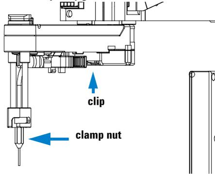
**3** Pull the capillary out off the capillary guiding pipe and out off the guiding hole in z-arm of the transport assembly.
