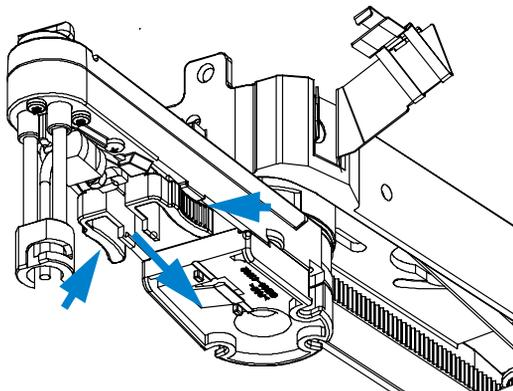
**3** Slide the new capillary guiding assembly into the holder of the capillary carrier assembly. Make sure to push it all the way to the front.
