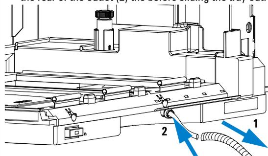
**4** Install the new tray by sliding it into position underneath the metal latch that holds it. The waste tubing from the internal tray should be guided as shown.
