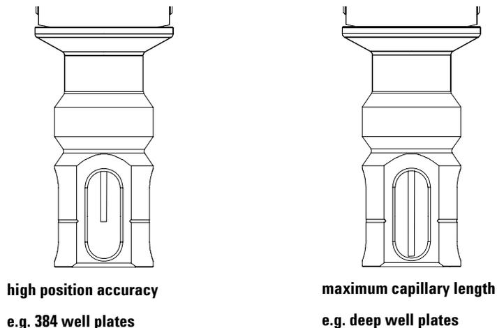
**Figure 3** Positions of the capillary tip
