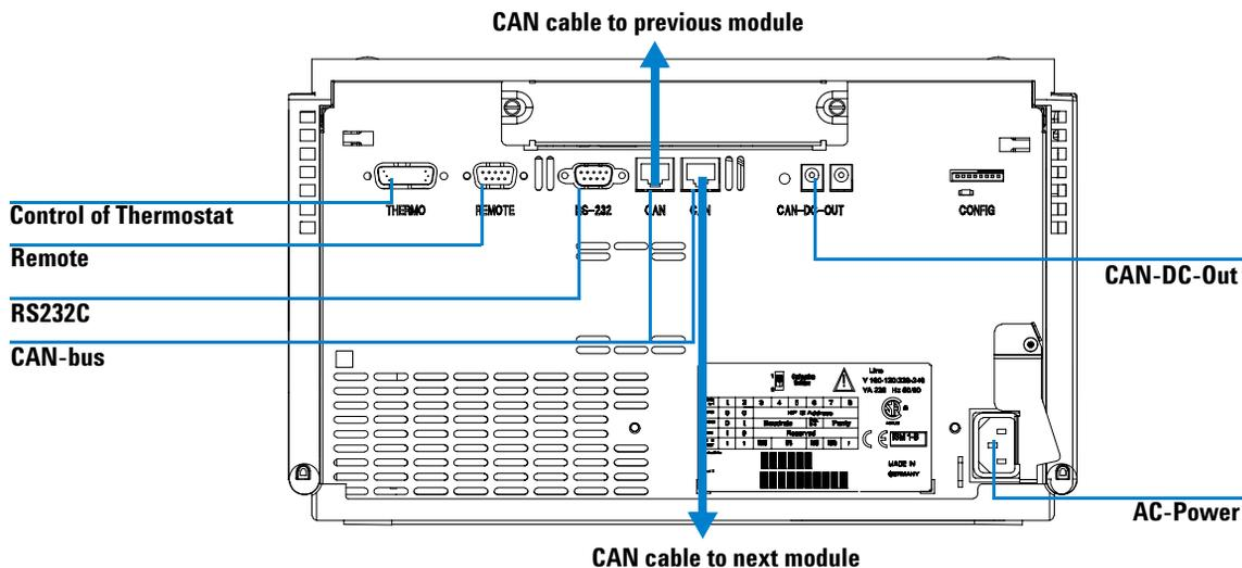
**Figure 3** Cable Connections
