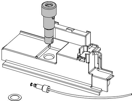
**4** After unscrewing the cap the waste port can be further disassembled.
