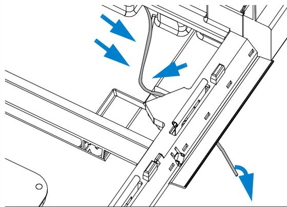
**5** Make sure that the waste tubing is slid all the way through the outlet (1). Its end should be over the edge and below the level of the laboratory desk that the system stands on to avoid any back flow of solvent. Re-install the corrugated waste tubing (2).
