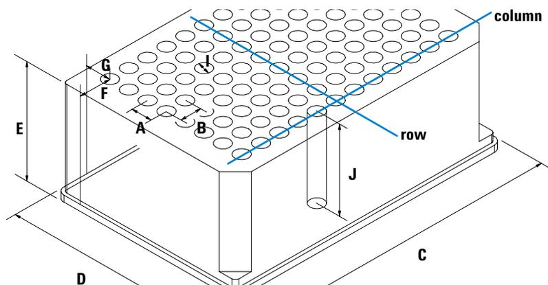
**Figure 7** Well-plate Dimensions (straight)
