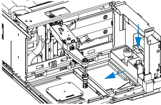
**2** Turn the tray upside down, unscrew the tubing and remove the washer.
