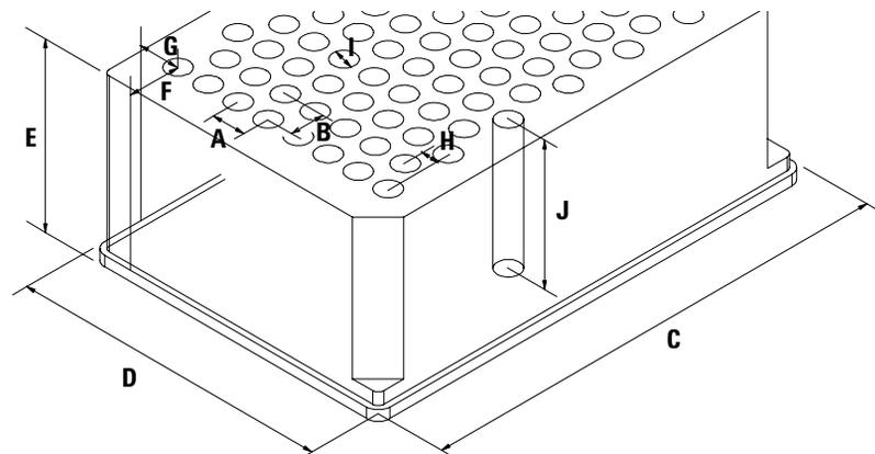
**Figure 8** Well-plate Dimensions (staggered)
