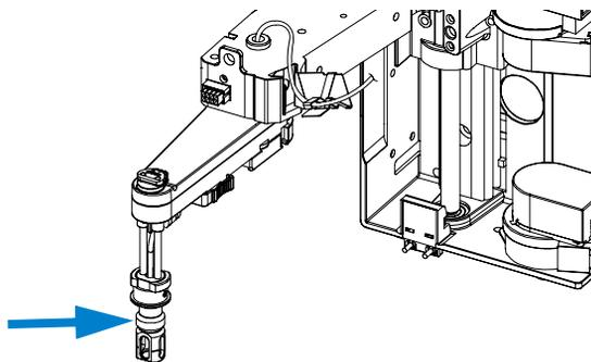
**2** Remove the clamp nut and remove the capillary from the clip at the bottom of the carrier assembly.
