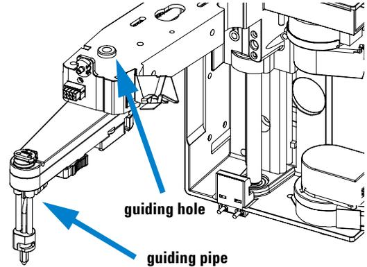
**4** Press the metal sheets of fixation spring together and push the capillary assembly out of the holder at the z-arm of the transport assembly.
