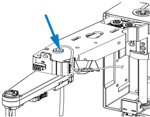
**7** Push the capillary through the guiding fitting assembly and attach the wellplate adapter. Then adjust the position of the capillary tip.
