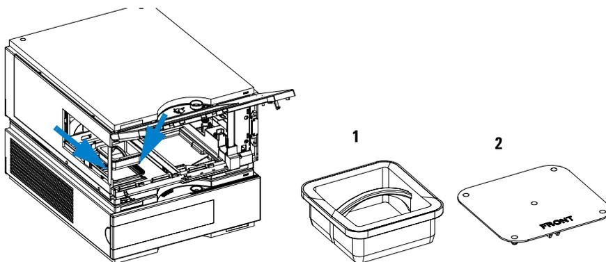
**Figure 4** Installation of Thermostat and Fraction Collector
