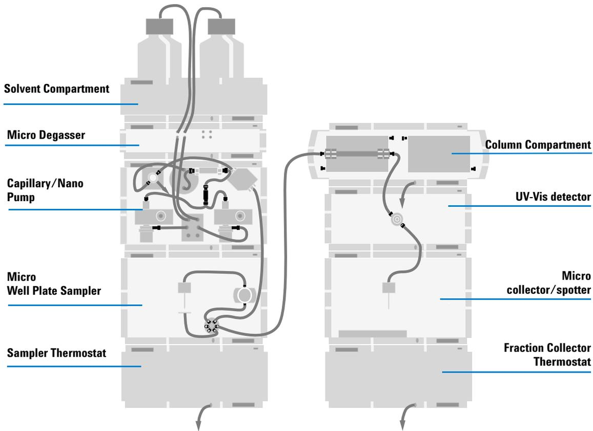
**Figure 1** Recommend Stack Configuration for micro-scale collector/spotter in the capillary or nanoflow system
