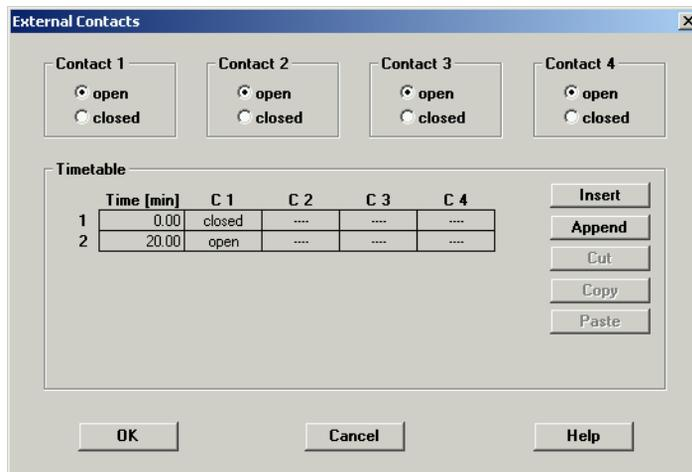
**Figure 15** Syringe Pump Control through External Contacts
