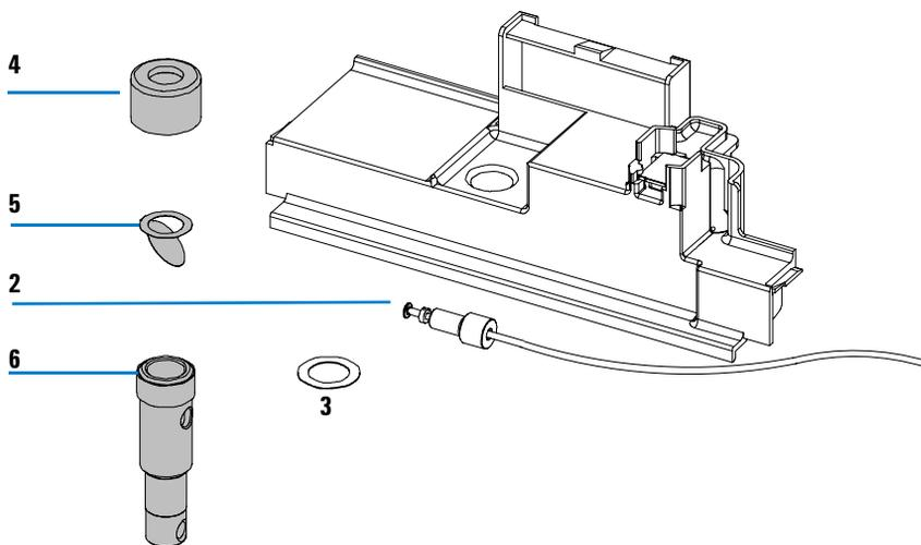
**Figure 24** Internal Tray Assembly (Micro Scale)
