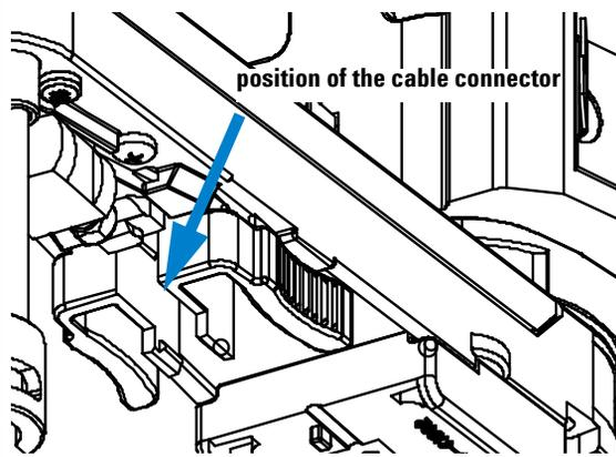
Exchanging the Micro-scale Fraction Collector/Spotter Lamp Assembly
