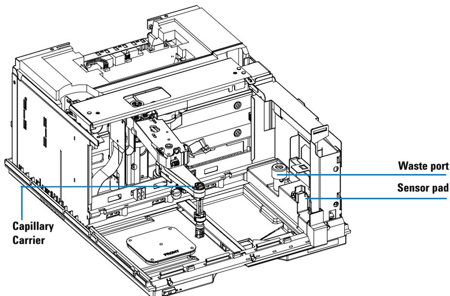
**Figure 1** The Agilent 1260 Infinity Micro-scale Fraction Collector/Spotter
