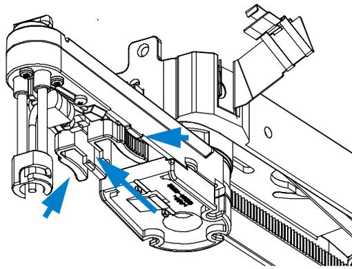
**4** Reinstall the Capillary, the clamp nut and the wellplate adapter.
