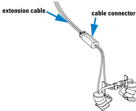
**5** To install the new lamp assembly unplug the connector as described in [step 4](#) and slide the cable from the top through the hole in the carrier assembly.
