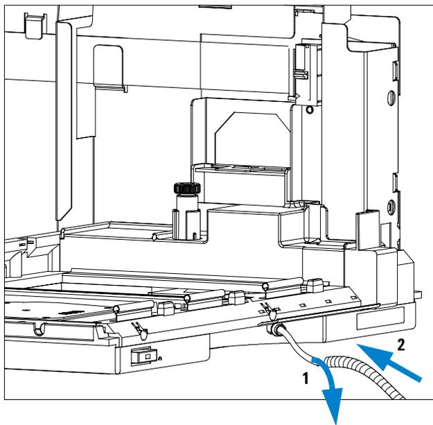
**Figure 2** Installing the Corrugated Waste Tubing in the Plastic Port
