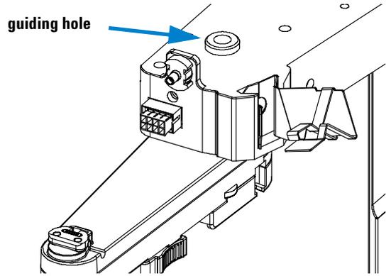
**6** Carefully bend up the two metal sheets of the lamp assembly, that hold the LEDs. Then slide the assembly onto the spotting adapter, that the t-shaped alignment plate fits into the slit between the pusher and the adapter.
