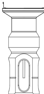
**8** If you are using a deep well plate, you should push the capillary through the guiding assembly, that the tip is close to the bottom of the wellplate adapter frame. The tip must stay within the oval frame.
