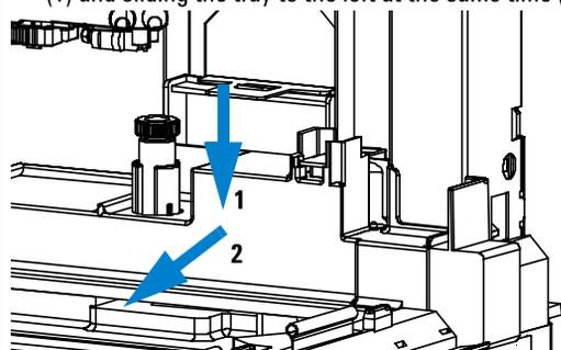
**3** Remove the corrugated waste tubing from the front of the instrument (1) and slide the internal tray's waste tubing to the rear of the outlet (2) before sliding the tray out.
