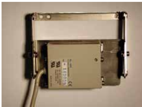
Figure 27 Barcode reader mounting position for landscape position
