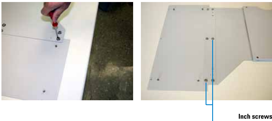
Figure 12 Assembling the sheet metal parts
