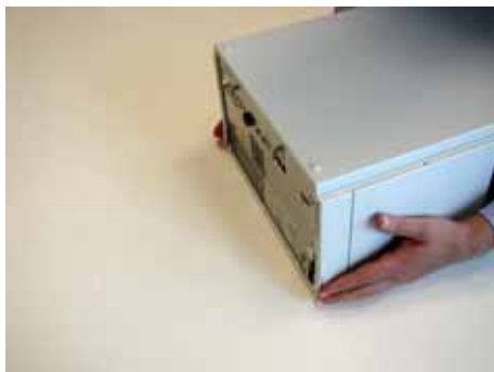
Figure 3 Removing the cover
