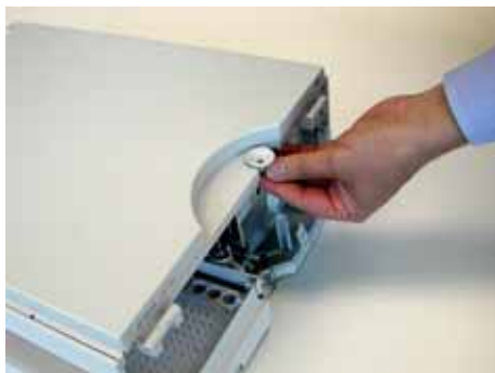
Figure 2 Removing the funnel
