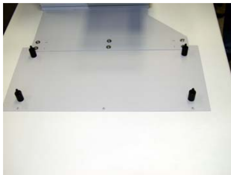
Figure 19 30 mm spacers (left) and mounted on the locating plate
