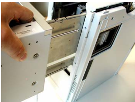
Figure 10 Moving the Automation Interface into the autosampler
