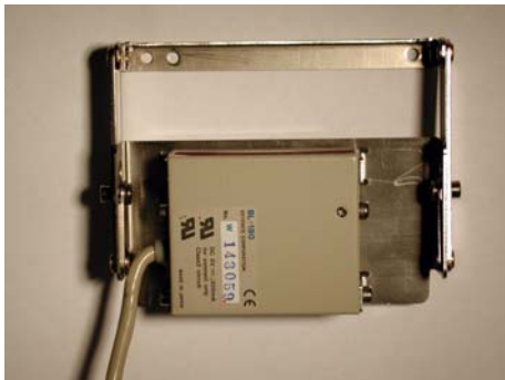
Figure 28 Barcode reader mounting position for landscape position
