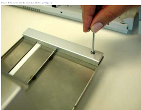
Figure 9 Removing the lock screw from the Automation Interface
