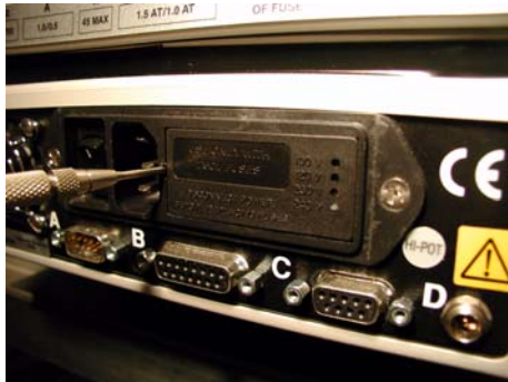
Figure 14 Prying open the cover/fuse-block assembly
