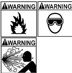
Risk of expelling fuel, oil vapors, hot steam, hot toxic exhaust gases, acid, refrigerant and other debris.
