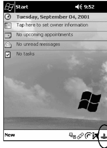
The default is to start the FTP Server at boot time, unless the following registry entry is defined and set to “0” which disables AutoFTP. “1” enables the AutoFTP. The entry can be set from the NDISTRAY pop-up menu by selecting either **AutoFTP On** or **AutoFTP Off**.
