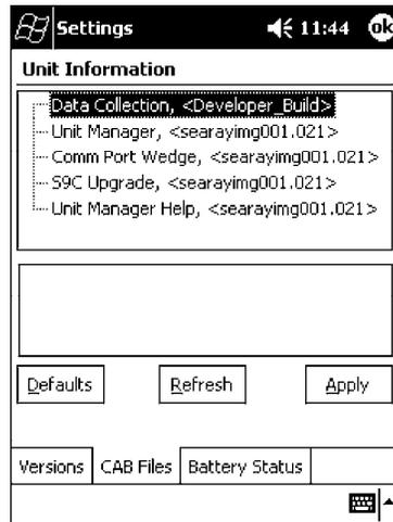
When a CAB file is built, a registry entry is created with a build number for that file. This CAB Files control panel applet looks for a registry key for each CAB file installed. When the registry entry is found, the CAB file name and version number information are displayed. If a CAB file has not been installed, then its information is not displayed.
