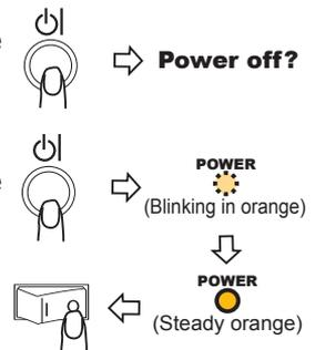
3. Make sure that the power indicator lights in steady orange, and set the power switch to the OFF position. The POWER indicator will go off. Attach the lens cover.
