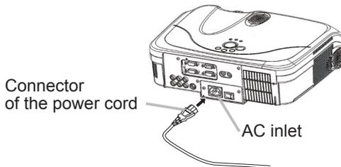
1. Connect the connector of the power cord to the AC inlet of the projector.
