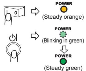
3. Press the STANDBY/ON button on the projector or the remote control. The projector lamp will light up and the POWER indicator will begin blinking in green. When the power is completely on, the indicator will stop blinking and light in green.
