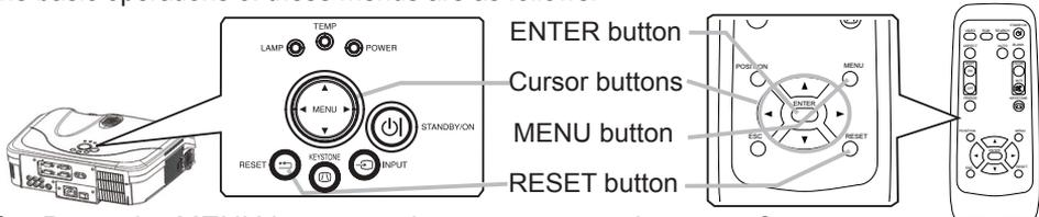
1. Press the MENU button on the remote control or one of the cursor buttons on the projector.
