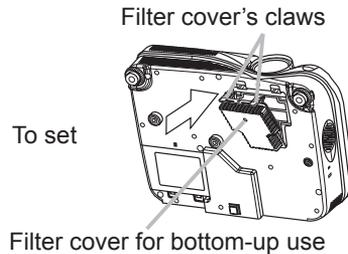
1. After making sure that the projector is cool adequately, slowly turn the projector so that the lens-side is facing up. Please be careful for the projector not to fall. While the projector is placed lens-side up, hold the projector.
