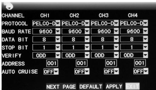
**Channel:** selecting the channel to which the PTZ camera is connected.
