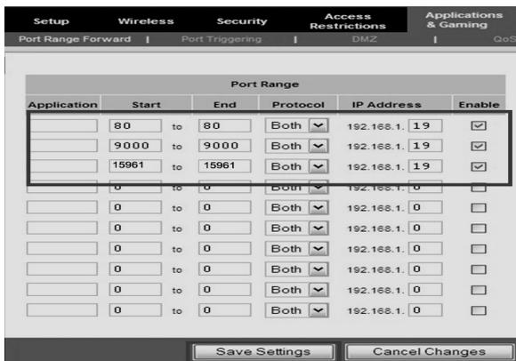
As shown above, fill in the IP and the port number in the corresponding files, and select “Both” in [Protocol]. The tick below [Enable] denotes “selected”. After setup, click “Save Setting” to save.
