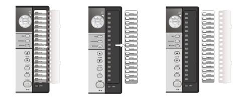
**O NOTE:** There is a replacement directory card in the telephone package. You can use it to replace the current one on the telephone if necessary.
