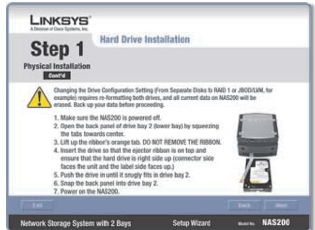
Physical Installation of the Second Hard Drive
