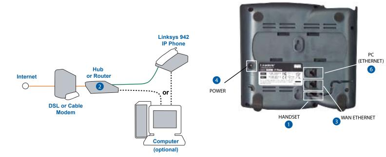
Step 1: Connect one end of the (RJ-11) spiral phone cord to the enclosed handset and the other end to the corresponding handset jack on the back of the phone. 1
