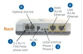
**Basic Installation Instructions** for connecting the ATA/router to the Internet via Cable or DSL modem
