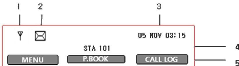
1. **Antenna** - Displayed when the LWS-WK is in the range of a LWS-BS where it can be linked. Disappears when it moves out of range. The closer it moves to the base, the stronger RSSI for reception is.
