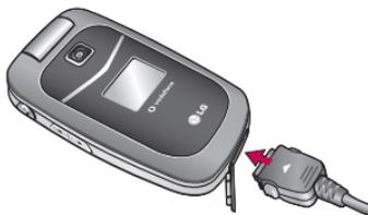
1. With the arrow facing you as shown in the diagram push the plug on the battery adapter into the socket on the left side of the phone until it clicks into place.
