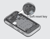
Use the stylus to press the reset key and hold it for a while. Your device may automatically restart and display the Home Screen.
