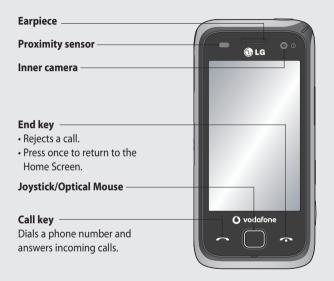
MARNING: Putting a heavy object on the phone or sitting on it can damage its LCD and touch screen functionality. Do not cover the protection film on the proximity sensor of the LCD as this can cause the sensor to malfunction.
