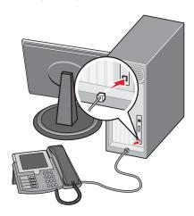
**5** Connect an additional telephone cord (not provided) from the computer modem to the printer EXT port  $\widehat{\mathbb{H}}$ .
