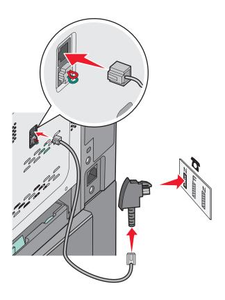
**3** Connect the adapter into the N slot of an active analog telephone wall jack.
