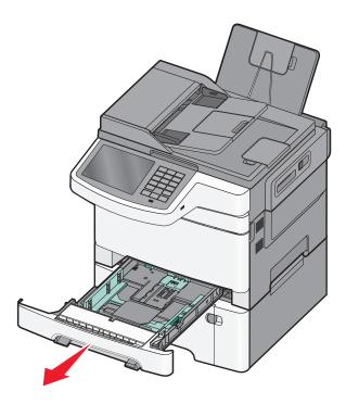
2 Squeeze the length guide tab, and then slide the guide to the correct position for the paper size being loaded.
