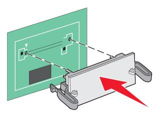
**Note:** The entire length of the connector on the card must touch and be flush against the system board.
