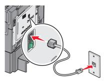
**3** Remove the plug from the printer EXT port :
