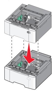
4 Align the printer with the 650-sheet duo drawer, lower the printer into place, and then install the dust covers.
