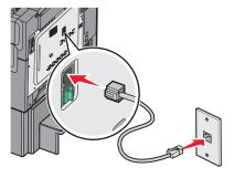
**3** Remove the protective plug from the printer EXT port  $\widehat{\mathbf{m}}$ .
