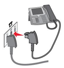
5 If you would like to use the same line for recording messages on your answering machine, then connect a second telephone cable (not provided) between the answering machine and the other N slot of the active analog telephone wall jack.
