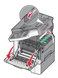
Remove the toner cartridges by lifting the handles, and then gently pulling away from the imaging kit.
