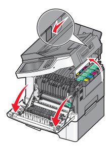
**3** Remove the toner cartridges by lifting the handles and then gently pulling away from the imaging kit.
