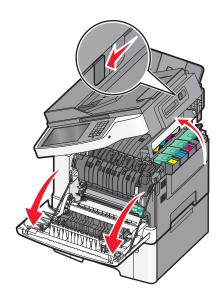
4 Remove the toner cartridge by lifting the handle, and then gently pull away from the imaging kit.
