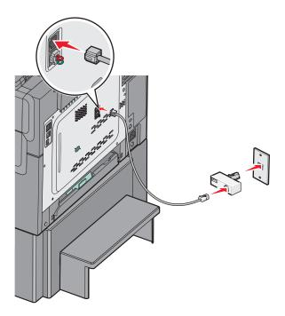
**3** Connect the answering machine or telephone to the adapter.
