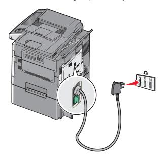
4 If you would like to use the same line for both fax and telephone communication, then connect a second telephone line (not provided) between the telephone and the F slot of an active analog telephone wall jack.
