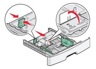
**Note:** Use the size indicators on the bottom of the tray to help position the guide.
