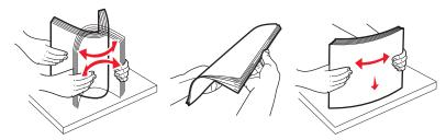
Hold transparencies by the edges, and then fan them. Straighten the edges on a level surface.
