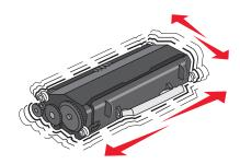
**5** Install the new toner cartridge by aligning the rollers on the toner cartridge with the arrows on the tracks of the photoconductor kit. Push the toner cartridge in as far as it will go. The cartridge *clicks* into place when correctly installed.
