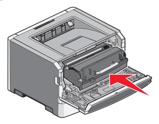
**8** After you replace the photoconductor kit, reset the photoconductor counter.
