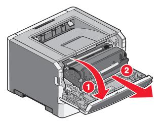
2 Lift the flap at the front of the printer, and then remove any jammed sheets of paper that are short lengths of paper.
