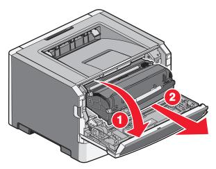
**2** Lift the flap in front of the printer, and then remove any jammed sheets.
