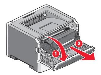
**4** Lift the flap in front of the printer, and remove any jammed sheets.
