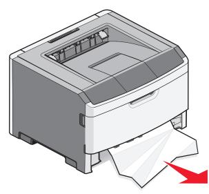
3 If you do not see it, open the front door, and then remove the photoconductor kit and toner cartridge (unit).Note: When the photoconductor kit and toner cartridge are together, they are called a unit.
