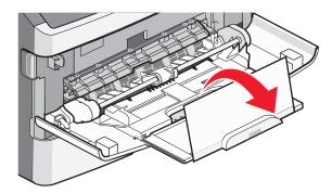
**4** Guide the extension down gently so the multipurpose feeder is extended fully and open.
