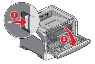
2 Press the button on the base of the photoconductor kit, and then pull the toner cartridge out using the handle.
