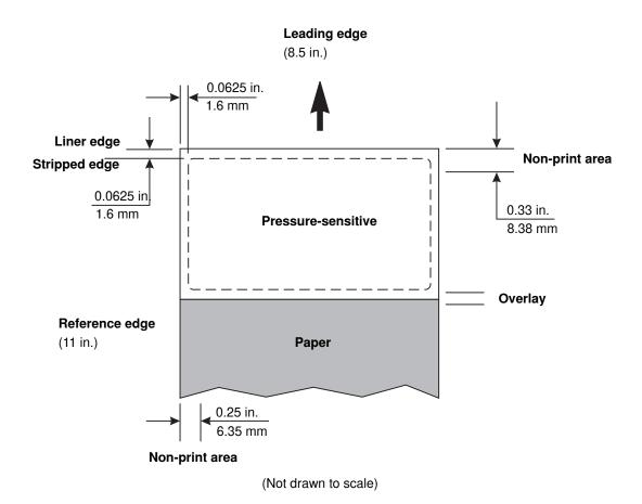
Figure 5. Design guidelines, dual web form
