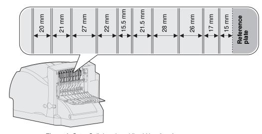
Figure 1. Optra S rib locations (rib width = 2mm)
