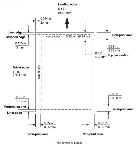
Figure 3. Design guidelines, vinyl label for Optra plus, 4039, 4029, and 4019 printers
