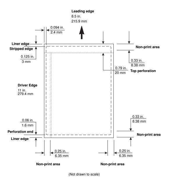
**Figure 4.** Design guidelines, vinyl label for Optra S, Optra T, and Lexmark T printers
