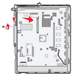
**Warning:** Option cards are easily damaged by static electricity. Touch something metal on the printer before you touch an option card.
