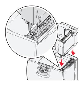
4 Attach the printer top cover to the output expander.
