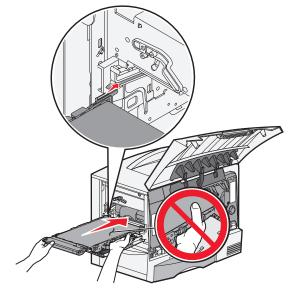
**b** Rotate the handle up, and push gently to lock the unit in place.
