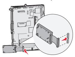
**8** Flip the hard disk over, and then press the three posts on the mounting plate into the holes on the system board. The hard disk *snaps* into place.
