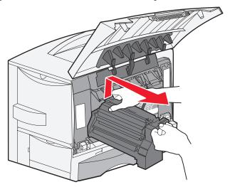
6 Release the latches to open the multipurpose feeder (area A) all the way.
