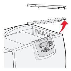
**Warning:** The output expander tray is designed to hold the weight of print material only. Do not use it as a shelf; excess weight may cause it to disengage from the output expander.
