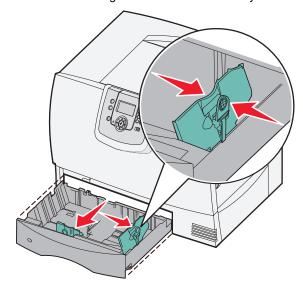
3 Squeeze the side guide lever and slide the guide to the correct position for the size paper you are loading. lcons along the back of the tray indicate paper sizes.
