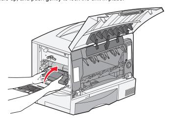
**c** Lower the lever to lock the image transfer unit into place.
