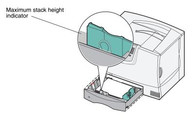
Note: Do not exceed the maximum stack height. Overfilling the tray may cause jams.
