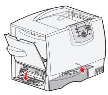
2 While holding down the front access door, insert a folded piece of paper as shown to clear the paper sensors under the image transfer unit. Make sure to clear the entire width of the paper path.
