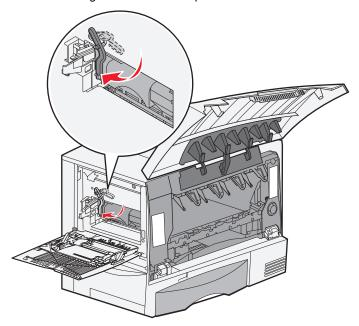
10 Return the multipurpose feeder to its working position.Reinstall all the print cartridges.
