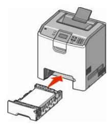
**7** If a different type of paper was loaded than the type previously loaded in the tray, then change the paper type setting for the tray from the printer control panel. For more information, see "Setting the paper size and type" on page 54.
