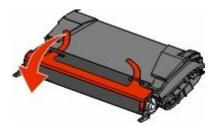
Insert the new cartridge into the printer.
