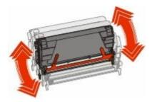
Remove the red packing strip from the new cartridge.
