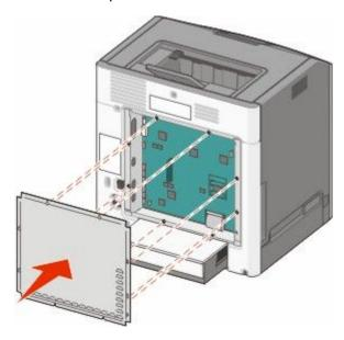
Slide the cover down, and then turn each screw clockwise to tighten.
