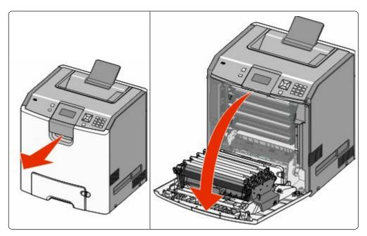
Pull up and out on the green tabs of the specified cartridge to remove it from the printer.
