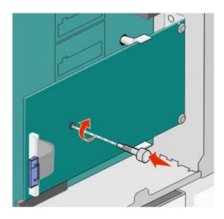
**9** Attach the two provided screws to secure the ISP mounting bracket to the system board cage.
