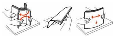
**5** Load the paper stack with the recommended print side faceup. Load the stack toward the back of the tray as shown.
