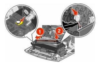
**5** Remove the red packing strip from the top of the photoconductor.
