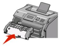
**b** Turn the screws to the right to fasten the fuser unit securely.
