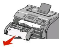
**d** Replace the fuser unit, and then turn the screws to the right to fasten it securely.
