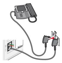
5 If you would like to use the same line for recording messages on your answering machine, connect a second telephone line (not provided) between the answering machine and the other N slot of the telephone wall jack.
