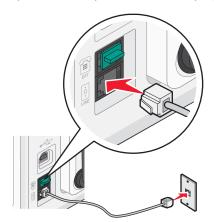
$\boldsymbol{3}$  Remove the protective plug from the EXT port  $\widehat{\;\;\square\!|\;}$  of the printer.
