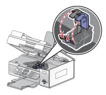
14 Remove the tape from the black print cartridge, and insert it in the left cartridge carrier.
