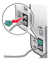
**4** Connect the other telephone cord to a telephone, and then plug it into the EXT port  $\widehat{\ }$  of the printer.
