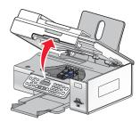
3 Press down on the cartridge carrier latch to raise the cartridge carrier lid.
