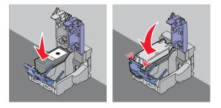
**16** Remove the tape from the color print cartridge, and insert it in the right cartridge carrier.
