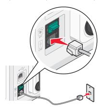
**3** Remove the protective plug from the EXT port  $\stackrel{\text{$\square$}}{}$  of the printer.
