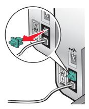
**4** Connect a second telephone cord from the computer modem to the EXT port  $\stackrel{\frown}{=}$  of the printer.
