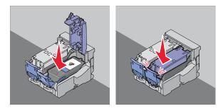
8 Close the printer, making sure to keep your hands out from underneath the scanner unit.
