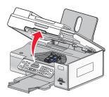
**2** Grasp the control panel at the front. Lift and rotate it back to remove it (if one is installed).
