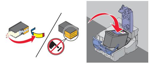
Warning: Do not touch the gold contact area on the back or the metal nozzles on the bottom of the cartridge.
