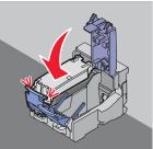
**6** Remove the tape from the back and bottom of the color cartridge, and insert the cartridge in the right carrier.
