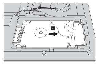
7 Take out the hard disk drive secured in a metal frame 5.
