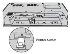
Out the battery back in place. Turn the computer over and reconnect the cables.
