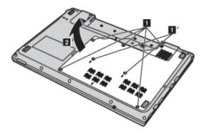
6 Remove the frame fixing screws 3.
