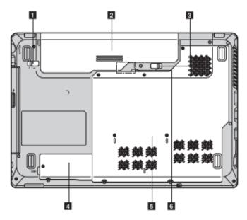
Battery latch - The manual battery latch is used to keep the battery pack secured in place.
