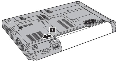
4. Unlock the battery latch **2** by sliding it to the unlocked position. While holding the latch **2** in the unlocked position, remove the battery **3**.
