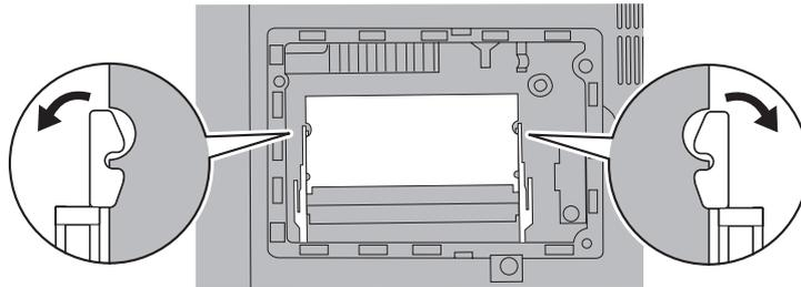
**Attention:** If only one SO-DIMM is installed, plug it into the SO-DIMM socket which is closer to the mainboard.
