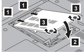
**Attention:** When you have added the SO-DIMM, do not use your computer until you have closed the memory slot cover. Never use the computer with the cover open.
