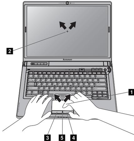
The blue indicator **5** is lit when the touch pad is activated, when the touch pad is disabled with Fn + F8, the indicator will be off.
