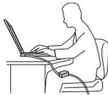
When the AC adapter is connected to an electrical outlet and your computer, it generates heat. Do not place the adapter in contact with any part of your body while using it. Never use the AC adapter to warm your body. Extended contact with your body, even through clothing, may cause a skin burn.
