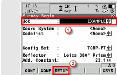
2. Initially, an existing Job must be selected, or a new one created. Select the Job field (1) to complete this task. Also, be sure to select the proper Coordinate System, Codelist, Config Set, etc.
