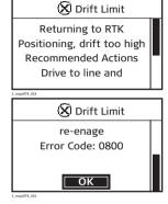
Press  $\binom{OK}{OK}$  to acknowledge and clear the error, drive to within the engage limits for the wayline and engage guidance.
