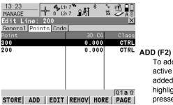
To add an existing point from the active job to the line. A new point is added before the point which was highlighted when ADD (F2) was pressed.
