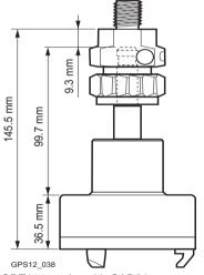
GRT144 carrier with GAD31 screw-to-stub adapter.
