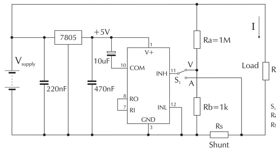
Measuring supply voltage and current to a load.
