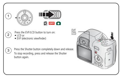
NOTE: After you take a video, the EVF/LCD displays a quickview for approximately 5 seconds.
