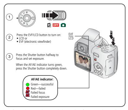
NOTE: After you take a picture, the EVF/LCD displays a quickview for approximately 5 seconds. The picture is saved unless you press the Delete button.
