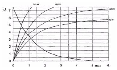
Figure 14. Heating and cooling curves for CEI OCX/65-G tube
