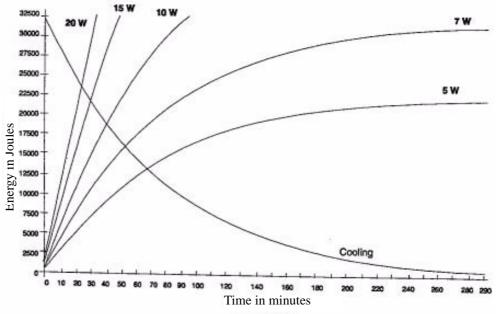
Figure 17. Heating and cooling curves of the KODAK 2100 system tube head
