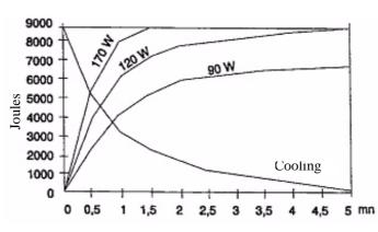
Figure 13. Heating and cooling curves for TROPHY TRX 708 tube
